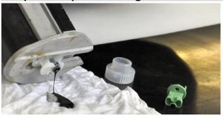
Push out some material <u>without</u> the mixing nozzle, to even out both pistons. Make sure both openings aren't plugged with hardened material.
