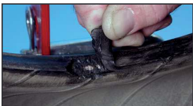
7. Deformed bead, exposed fabric or steel
