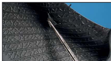
10. Tire damage from impacts
