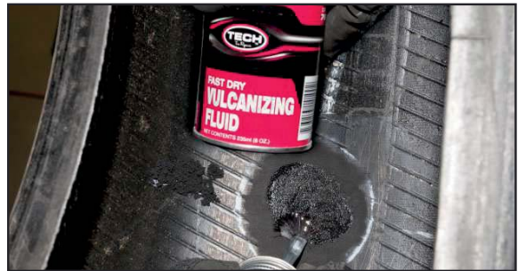
13. Apply a thin, even coat of Chemical Vulcanizing Fluid #760 or Heavy Duty Blue Vulcanizing Fluid #775 to the buffed surface. Allow 3-5 minutes drying time for #760 or 5-8 minutes for #775. Additional drying time may be required in adverse weather conditions.
