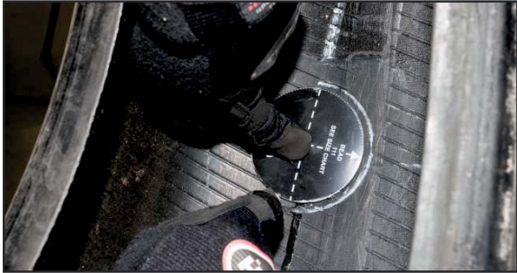
10. Outline the area to be buffed 1/2" (13mm) larger than the repair being used, or use the appropriate repair template.
