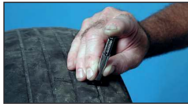
5. Excessive tread wear
