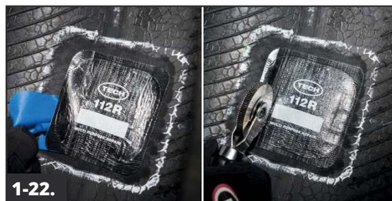
**1-22.** Remove the poly from under the repair unit and continue stitching from the center out, using firm pressure.
