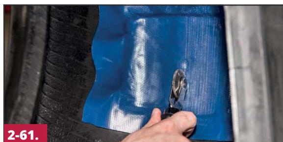
Place the cushion gum over the buffed area and stich the cushion gum from the center out. Be sure not to trap air in the transition area between the casing and the inner liner.
