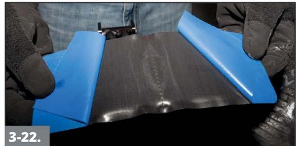
**3-22.** Break the perforation in the blue poly on the back of the repair unit. Peel the poly back on both sides to expose the center of the repair unit's cushion gum, while leaving the edges covered. Use the poly to grasp the repair unit and prevent contamination of the cushion gum.
