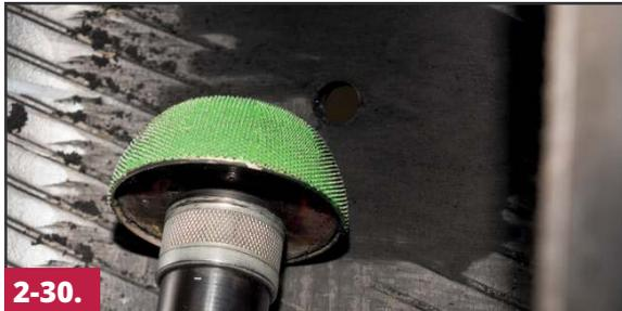
Using a fine grit buffing wheel (#RH107 or #FCRT3CR50 or equivalent) on a low RPM buffer (5,000 RPM Max.), buff an area approximately 1 ½" (40mm) in all directions around the injury.
