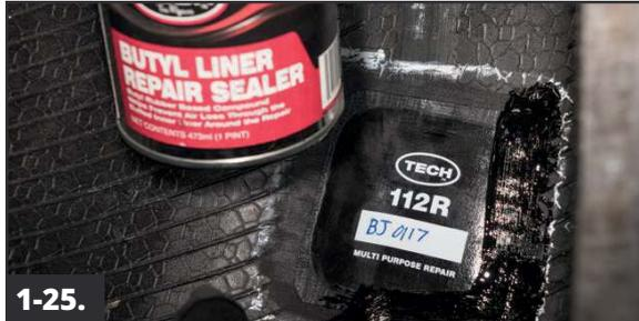
Apply Butyl Liner Repair Sealer #739 to the edge of the repair unit and to the overbuffed surface on the inner liner to retain proper air retention.
