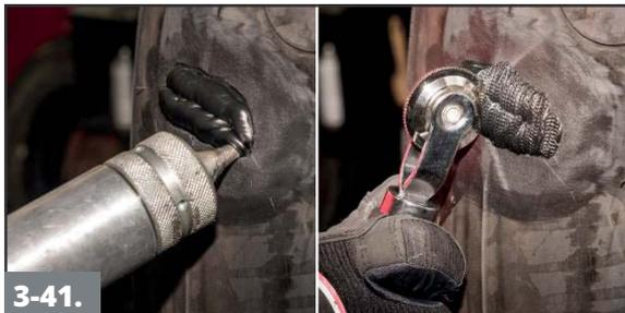
**3-41.** Finish filling the cavity with rope rubber until the rubber is built up 1/8" (3mm) above the tire's surface. Stitch the rubber using firm pressure to remove trapped air. The tire is now ready for curing.
