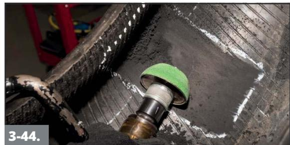
**3-44.** Using a fine grit buffing wheel (#RH107 or #FCRT3CR50 or equivalent) on a low RPM buffer (5,000 RPM max.), buff the inner liner area marked to a #1 or #2 buffed texture, being careful to stay within the marked area.
