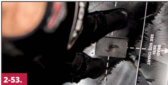
Use the appropriate size repair template and a tire crayon to mark the area where the inner liner is to be removed. If a template is not available, mark an area at least 1/2" (13mm) larger than the repair unit being installed.
