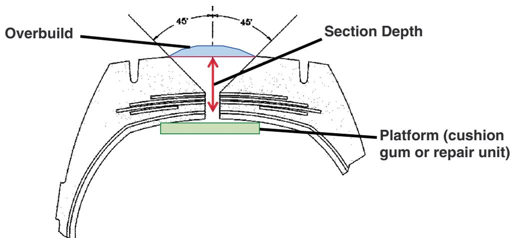
To determine the cure time measure the section depth (thickness of the tire at the deepest point of the skive). Then add this to the thickness of the repair and overbuild of the filler rubber. The total thickness is then multiplied by the cure rate of the rubber being used. **This does not include equipment warm up time.**
