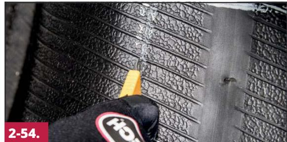
Use a sharp knife #807 to cut the inner liner along the outer perimeter of the outlined area. Lift the edge of the inner liner with the knife or a probe to determine the thickness of the material to be removed.
