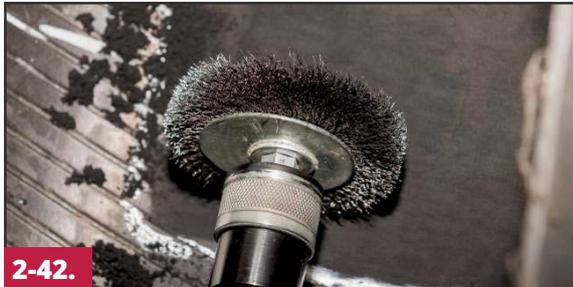
Clean the buffed area on both inside and outside of the tire using a soft wire brush (#S892) on a low RPM buffer. Remove the buffing dust by lightly brushing the buffed area from the right side to the left. Repeat the process a minimum of 2 - 3 times to ensure that all buffing dust is removed.
