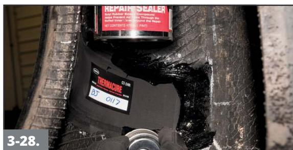
3-28. Apply Butyl Liner Repair Sealer #739 or Security Coat #738 to the edge of the repair unit as well as any buffed surface beyond the edge of the repair unit.
