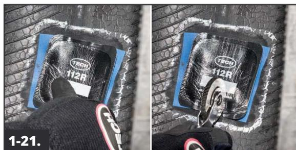
**1-21.** Press down the center of the repair unit with your thumb. Begin stitching from the center outward, using firm pressure. Stitch out to the folded poly.
