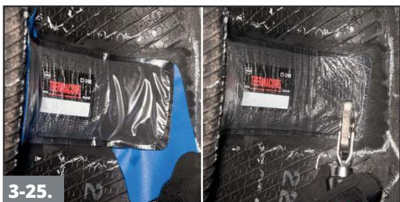
3-25. Remove the blue poly from under the repair unit and continue stitching outward using firm pressure.
