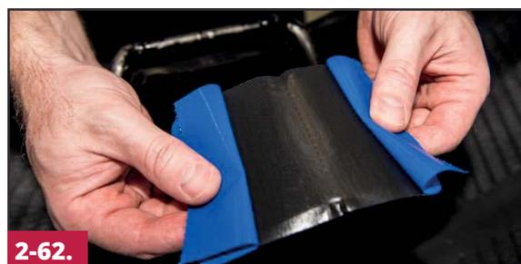
Break the perforation on the back of the repair unit and expose the center of the repair, leaving the protective poly on both ends.
