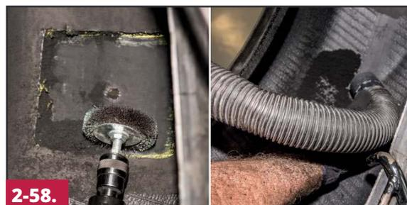
Use a soft wire brush moving from right to left to remove buffing dust and debris from the buffed area. Use a vacuum to remove this material from the tire.
