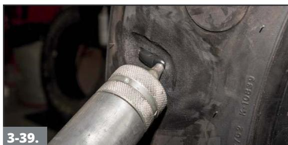
**3-39.** Pre-heat the extruder gun. Exerting firm pressure on the extruder, apply TRRP or LRRP rope rubber into the injury channel from the outside of the tire.
