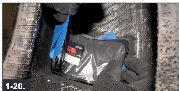
**1-20.** If the injury is a Reinforced Shoulder Repair, fold the repair unit, and then position the repair unit so that it is completely within the buffed area, aligning the bead arrows to the tire's beads. Release the repair unit and check the alignment. If the repair unit is not straight and/or completely within the buffed area, lift the repair unit and reposition.
