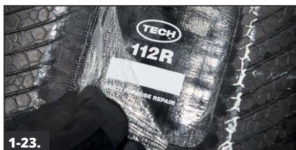
**1-23.** Remove the clear poly from the top of the repair unit and inspect the repair unit for trapped air. If trapped air is found, stitch the repair unit again until all trapped air is removed. If the trapped air cannot be removed, remove the repair unit and return to step 1-18 and install a new repair unit.
