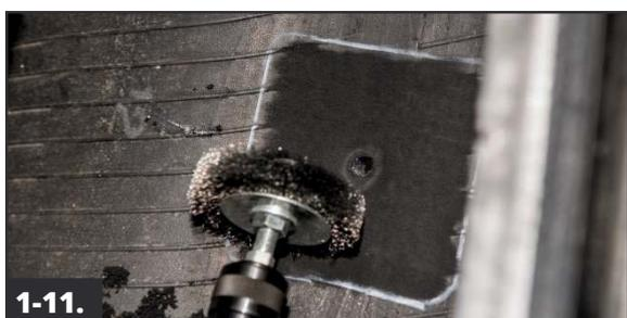
Clean the buffed area using a soft wire brush on a low speed buffer. Remove buffing dust by lightly brushing from the right side of the buffed surface to the left side. Repeat until all dust is removed.
