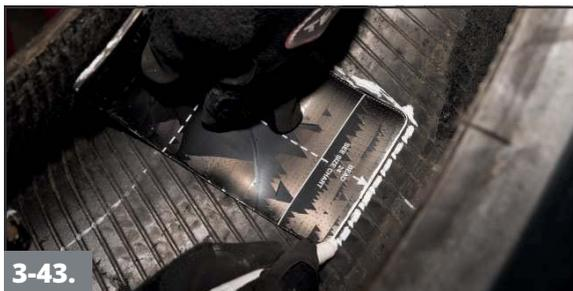
**3-43.** Use the appropriate size template and a tire marker to mark an area on the inner liner for buffing. When placing the template be sure to place the lines for the reinforcement package outside of the flex area of the tire.
