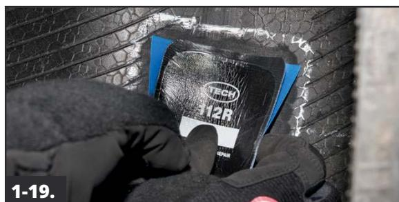
**1-19.** Fold the repair unit and position the repair unit, aligning the beads arrows to the tire's beads if a reinforced repair is being used. Center and place the repair unit over the injury. Release the repair unit to check for proper placement and alignment. If the repair unit is not centered and/or straight, lift the repair and reposition.
