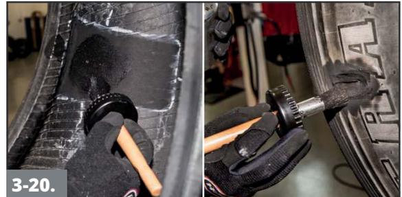
**3-20.** If installing a Thermacure repair, apply a thin, even coat of TemVulc black cement to the buffed inner liner and skive areas. If installing the repair unit chemically, use Chemical Vulcanizing Fluid. **Cement Drying Times:** TemVulc: 8-10 minutes; Chemical Vulcanizing Fluid: 3-5 minutes; Heavy Duty Blue Vulcanizing Fluid: 5-8 minutes. Additional time is necessary in cold and/or humid conditions.
