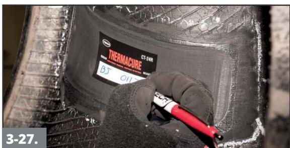
3-27. Mark the date and retread plant DOT code (if applicable) onto the repair unit with a dark or silver ink pen.
