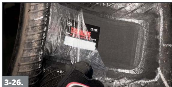
3-26. Remove the clear poly from the top of the repair unit and inspect the repair unit for trapped air. If trapped air is found, stitch the repair unit again until all air is removed. If the trapped air cannot be removed, remove and install a new repair unit.
