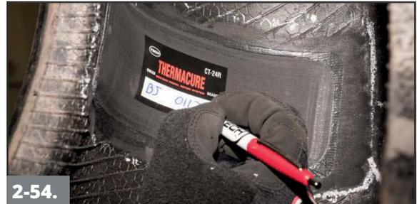
Use a dark ink pen or marker to mark the date and retread plant DOT code (if applicable) onto the repair unit.
