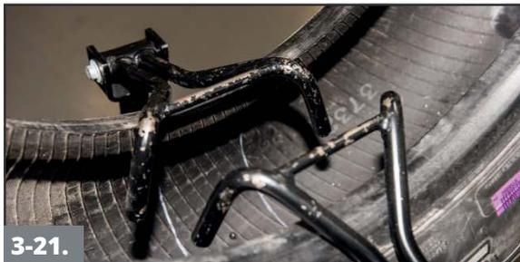
**3-21.** Release the spreader so that the beads of the tire are in a relaxed position prior to installing the repair unit. This will help prevent bridging of the repair unit.
