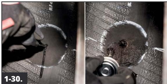
Using a spiral cement tool, apply Chemical Vulcanizing Fluid #760 into the injury 3 to 5 times to ensure the cement is coating the entire injury channel. Leave the cement tool in the injury after the last application. Next, apply a thin, even layer of Chemical Vulcanizing Fluid to the entire buffed surface. Allow 3-5 minutes for Chemical Vulcanizing Fluid to completely dry. Additional drying time will be needed in cold or humid conditions.
