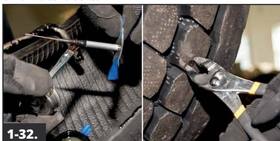
Apply Chemical Vulcanizing Fluid to the tapered part of the stem only and insert the lead wire through the injury from the inside of the tire. Grasp the wire with pliers on the outside and pull the stem through the tire until the cap forms a slight indentation. Do not over pull the stem.
