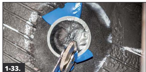
Press down the repair with your thumb, working from the center out. With the poly still in place under the cap, stitch the repair from the center out using firm pressure.
