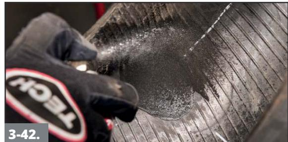
**3-42.** After the tire is cured and has cooled to room temperature, pour or spray Rub-O-Matic #704 or 704A or Citrus Based Rubber Cleaner #705C on the inner liner and use a #933 scraper to clean the inner liner. Repeat this process 2-3 times to remove any foreign materials that might contaminate the repair area or buffing tools.
