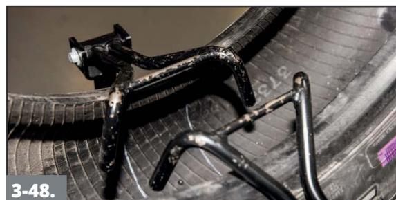
Once the cement is dry, release the spreader so that the tire is in a relaxed position prior to installing the repair unit. This will reduce the risk of bridging the repair unit.
