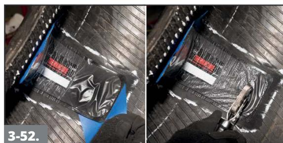
Remove the poly from under the repair unit and continue stitching from the center toward the edges of the repair unit.
