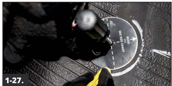
Center the appropriate repair template and use a tire crayon to mark the area on the inner liner for buffing. If a template is not available, center the repair unit over the injury and mark an area approximately 1/2" (13mm) larger than the repair unit.
