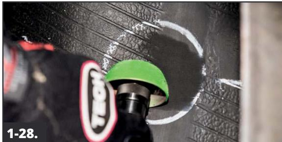
Using a fine grit buffing wheel on a low RPM air buffer (5,000 RPM max), buff the marked area on the inner liner to a #1 or #2 buffed texture, staying within the marked area.
