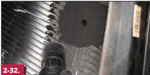
Vacuum all of the buffing dust from the tire. Do not touch the buffed surface with the vacuum as this could lead to contamination.
