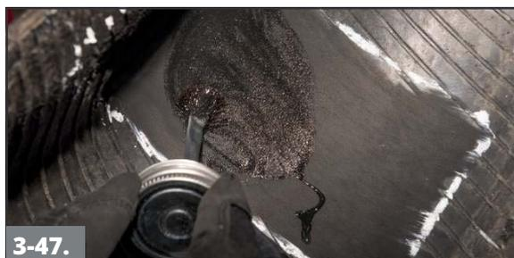
Apply a thin, even coat of cement by stippling the cement onto the inner liner. Cement the tire by applying a thin, even coat of cement by stippling the cement onto the inner liner. Use Chemical Vulcanizing Fluid #760 or Heavy Duty Blue Vulcanizing Fluid #775 for cold, or chemical cure applications. Allow the cement to dry thoroughly.
