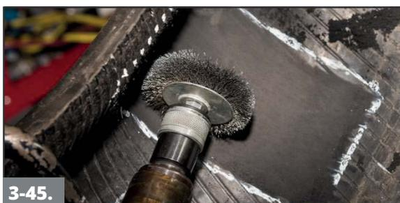
**3-45.** Clean the buffed area on both inside and outside of the tire using a soft wire brush on a low RPM buffer. Remove the buffing dust by lightly brushing the buffed area from the right side to the left. Repeat the process a minimum of 2 – 3 times to ensure that all buffing dust is removed.
