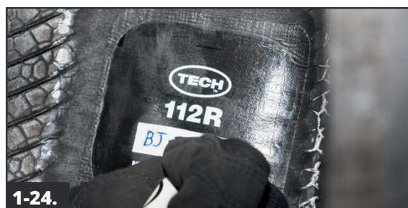
**1-24.** Initial and date the repair unit with a tire marker or silver ink pen for proper tracking.
