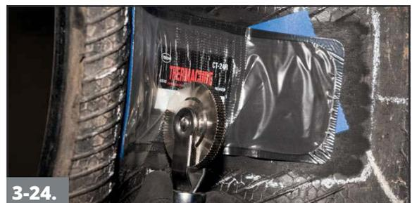
**3-24.** Press down the center of the repair unit. Begin stitching the repair unit from the center outward using firm pressure. Stitch the repair unit out to the folded poly.
