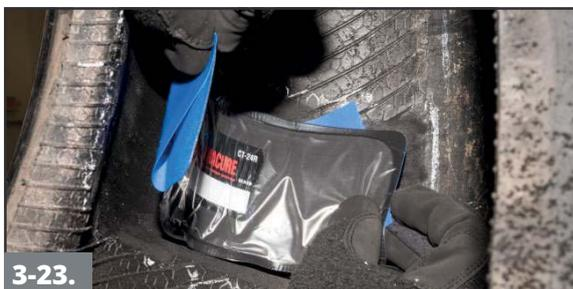
**3-23.** Fold the repair unit, then position the repair unit over the buffed surface, aligning the bead arrows toward the tire's beads. Place the repair unit over the injury and check the alignment. If the repair unit is not straight and/or properly positioned within the buffed surface, lift the repair unit and reposition.
