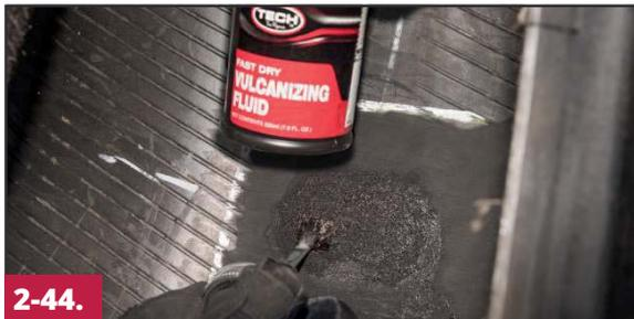
Apply a thin, even coat of cement by stippling the cement onto the inner liner. Use Chemical Vulcanizing Fluid #760 or Heavy Duty Blue Vulcanizing Fluid #775 for cold, or chemical cure applications. Allow the cement to dry thoroughly.
