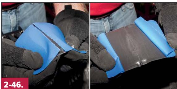
Break the perforation in the poly and peel back the poly approximately half way to expose the center of the repair unit's cushion gum. Use the poly to grasp the repair unit and keep the cushion gum clean.
