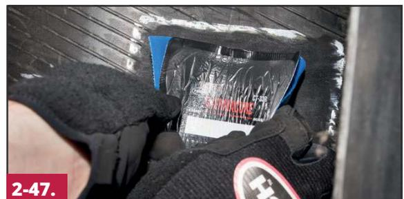
Fold and position the repair unit so that the repair unit's bead arrows are pointed toward the tire's beads. Center the repair unit over the injury and place the center of the repair unit against the inner liner. Release the repair unit and check that the repair unit is properly aligned and centered. If the repair unit is not centered, and/or straight, lift and reposition the repair unit.
