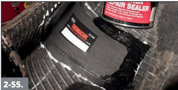
Apply Butyl Liner Repair Sealer #739 or Security Coat #738 to the edge of the repair unit as well as to any buffed surface not covered by the repair unit. Allow the tire to sit for 24 hours before returning to service.
