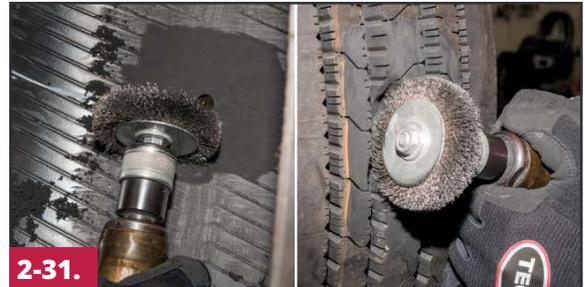
Clean the buffed area on both inside and outside of the tire using a soft wire brush on a low RPM buffer. Remove the buffing dust by lightly brushing the buffed area from the right side to the left. Repeat the process a minimum of 2 - 3 times to ensure that all buffing dust is removed.
