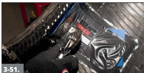
Press down the center of the repair unit with your thumb or the side of your hand. Begin stitching the repair unit from the center out, using firm pressure. Stitch out to the folded poly.
