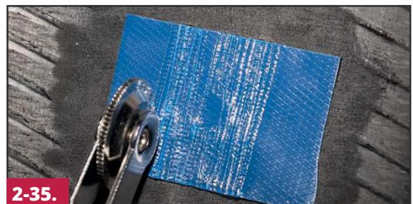
Apply the Vul-Gum to the buffed area on the inner liner. Stitch the Vul-Gum from the center out. Remove the poly from the Vul-Gum after it is thoroughly stitched.
