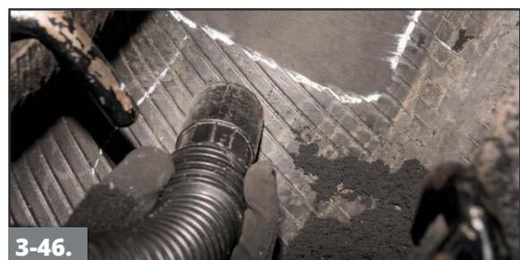
**3-46.** Vacuum all of the buffing dust from the tire. Do not touch the buffed surface with the vacuum as this could lead to contamination.
