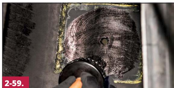
Apply a thin, even coat of Temvulc Black Cement #1082 to the entire buffed surface on both the inside and outside of the tire. Allow 8-10 minutes drying time. Additional time will be necessary in cold or humid conditions.
