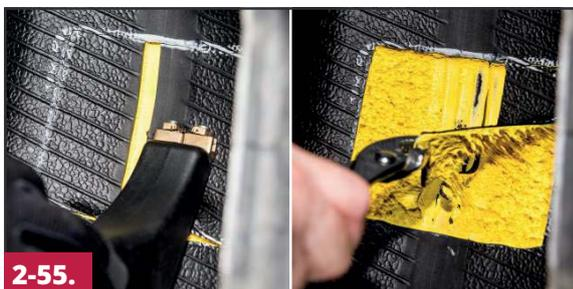
Using a tire regroover with a wide flat blade (W-5 or W-6 style) set to the appropriate depth, cut the inner liner and sealant material out of the tire in the outlined area, leaving a thin layer of the sealant on the casing. An alternative method is to completely remove the cut inner liner by pulling it out with a pair of pliers before using the regroover to remove the sealant material.
