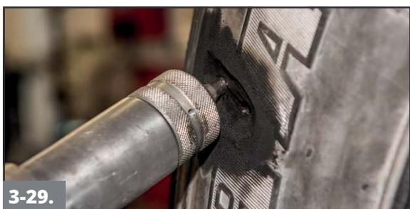
3-29. Using a preheated extruder, apply rope rubber into the cavity while exerting firm pressure with the extruder to prevent trapping air.
