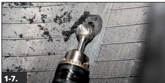
Using a small ball rasp, remove a small area of the inner liner around the injury to inspect the casing. If splits in the rubber and/or loose cables are detected, the damage must be removed. This can be accomplished by using a larger carbide cutter. If the damage is still within puncture limitations, then proceed to the next step. If not, then proceed to the Crown Section Repair procedures on page 10 of this manual.
