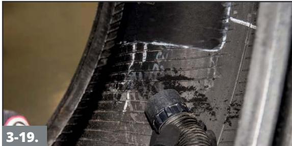
**3-19.** Vacuum all of the buffing dust from the tire. To avoid contamination, do not touch the buffed surface with the vacuum.
