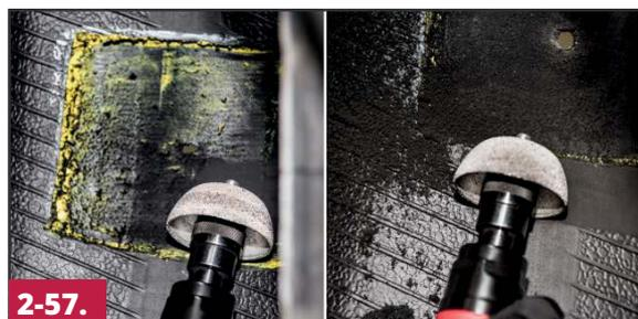
Once the sealant material has been completely removed from the casing, buff the exposed area of the casing with a fine grit buffing wheel (RH107, FCRT3CR50 or equivalent) on a low RPM buffer to a #1 or #2 buffed texture. Also, buff a 1-1/2" (40mm) area on the inner liner on all sides of the exposed area with the buffing wheel rotating inward toward the cut edge of the inner liner.
