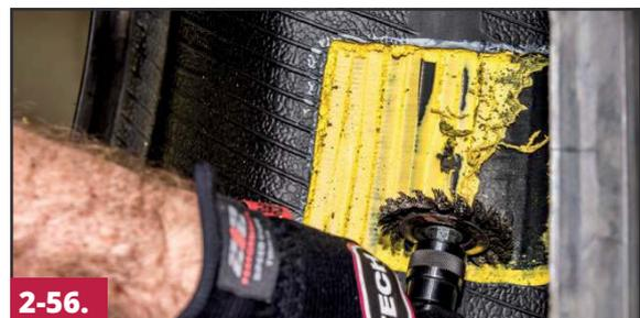
Using a twisted wire brush on a low RPM buffer, lightly buff the remaining sealant material from the exposed area. Make sure to completely remove the sealant material from the edges and corners where the inner liner has been cut away.
