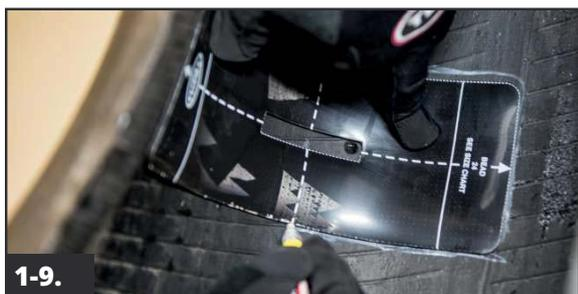
If the injury is in the outer 1.5" (40mm) of the tread, process the injury as a Reinforced Shoulder Repair. Select the appropriate size template. Position the template over the injury so the template is shifted toward the bead, keeping the injury within the template window. This will ensure that the fabric reinforcement in the repair unit extends beyond the high flex area of the tire.
