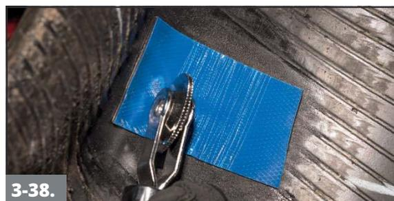
**3-38.** Apply the Vul-Gum to the buffed area on the inner liner. Stitch the Vul-Gum from the center out. Remove the poly from the Vul-Gum after it is thoroughly stitched.
