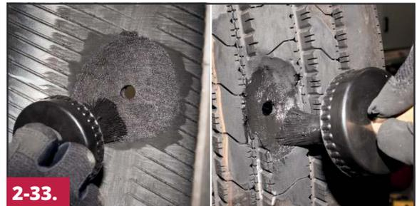
Apply a thin, even coat of Temvulc Black Cement #1082 to the buffed surfaces on both the inner liner and the outside skive. Allow to dry 8-10 minutes. More drying time may be necessary in cold and/or humid conditions.
