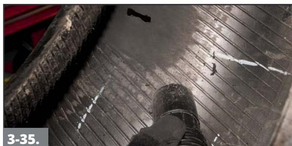
**3-35.** Vacuum all of the buffing dust from the tire. Do not touch the buffed surface with the vacuum as this could lead to contamination.
