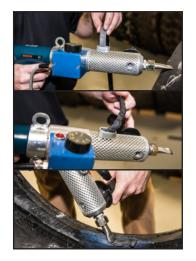
7. It may be necessary to process the A & B strip rubber material through the extruder tool a second time to ensure proper mix. During the second pass, if required, extrude the mixture into the injury, over lapping a layer at a time until the skive is completely filled.
