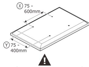
If width  $\bigotimes$  is greater than 600mm or height  $\bigotimes$  greater than 400mm STOP installation now and contact the customer help line
