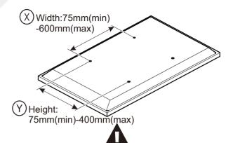
If width  $\bigotimes$  is greater than 600mm or height  $\bigotimes$  greater than 400mm STOP installation now and contact the customer help line
