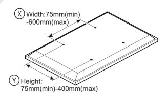
If width  $\bigotimes$  is greater than 600mm or height  $\bigotimes$  greater than 400mm STOP installation now and contact the customer help line
