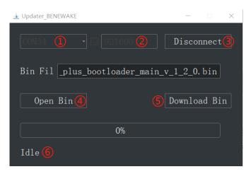
Figure 6: Firmware Upgrade PC software of TF-Luna
