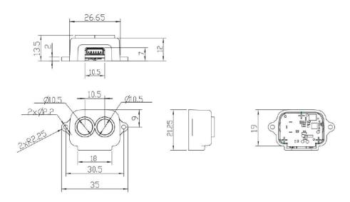
Figure 3: Constructional Drawing of TF-Luna
