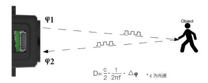
Figure 1: Schematics of TOF Principle
