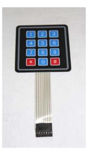
Punch in your secret key into this numeric matrix keypad. This keypad has 12 buttons, arranged in a telephone-line 3x4 grid. It's made of a thin, flexible membrane material with an adhesive backing (just remove the paper) so you can attach it to nearly anything. The keys are connected into a matrix, so you only need 7 microcontroller pins (3-columns and 4-rows) to scan through the pad. Check the tutorials tab for links to an Arduino library and example code.
