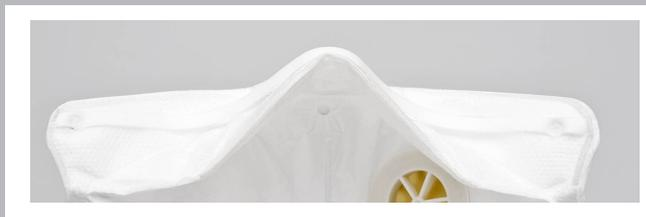
In order to reduce the chance of product contamination (required by various industries among which the pharmaceutical and the food industries), the internal nose clip is set between two layers of fabric to reduce as much as possible the aluminum parts of the PPE.
