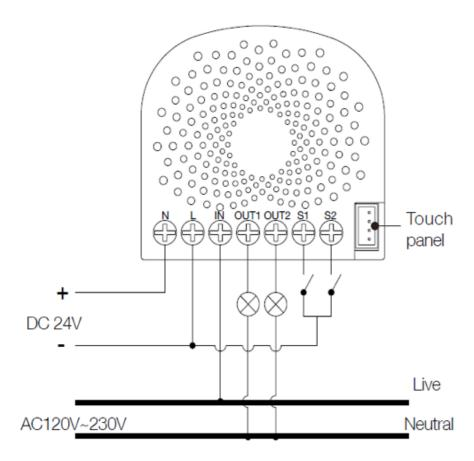
Note: The ?IN? terminal should be connected to the ?Live? of AC 120V/230V power wire.
