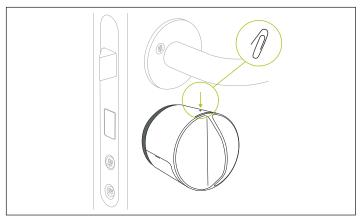
3) The *Click Command* configurations are executed via the small hole in the top of the Danalock V3. Use a paper clip or other suitable device to perform the clicks.
