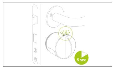
5) After 5 sec the lock confirms the choice and the configuration will begin. During the setup the LED blinks *white*. It will stop blinking when the calibration is done.
