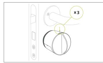
4) To activate the *automatic calibration* you have to click/ press three times through the hole.
