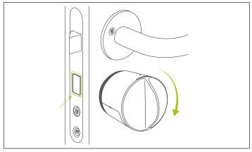
2) Make sure the door is unlocked. If it's not, turn the lock to unlocked position. Close the door.
