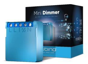
The Qubino Mini Dimmer is 25% smaller than any other wireless dimmer in the world. Mini Dimmer is a MOSFET-switching light device that also supports control of low-voltage halogen lamps with electronic transformers, dimmable compact fluorescent lights, and dimmable LED bulbs. It can work with or without the neutral line (3 or 2-wire installation).
