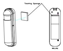
After finish the test and decide to fix, then you can remove tape A, and mounting the sensor by using tape B. The tamper key will pressed and let the sensor normal mode.
