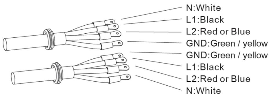
**In regards to IEC 60446 wiring color mark standards in the EU where only Neutral, L1, and Ground are present (L2 and L3 do not exist for the EU model):**
