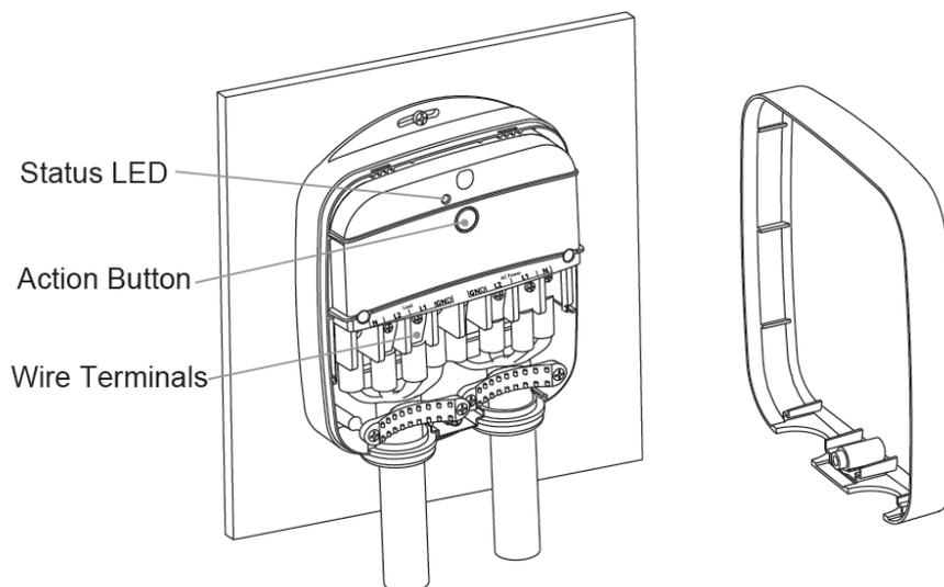
**Action button:** Used for Heavy Duty Smart Switch Z-Wave network inclusion and exclusion and to manually turn on or off.
