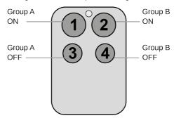
4 Groups are controlled with two buttons and double click (parameter 1/2 = 2) This mode enhances the previous mode and allows to control two furth-groups C and D using double clicks.
