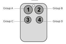
2 Groups are controlled with two buttons (parameter 1/2 = 1) The buttons 1 and 3 control the control group A (button one turns on, button three turns of buttons 2 and 4 control the control group B (button two turns on, button four turns off). In case dimmers are controlled, holding down the larger button will diholding down the smaller button will dim down the load. Releasing the button will stop the dimming function.
