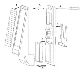
The siren can be placed on every location outside the home. Thanks to rating IP56 the location does not even need to be dry but please make sure it is placed high enough so that children do not accidently remove it. The device is self-protected against tamper and theft. In a first step the mounting plate (isee illustration above) is placed on the wall using the 4 screws provided. It is recommended to mount the complete device 5 mm from the wall for better sound.
