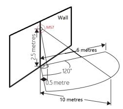
There are some placement considerations when using the Multisensor 7 as a motion sensor. Above are some diagrams that show the distance at which the wall or ceiling installations can perform based on the height they are installed at and at the angle.
