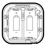
**Note:** MultiSensor 7 can be powered by a single CR123A (doesn't matter which port), though batteries will require changing more frequently (half the expected battery life).
