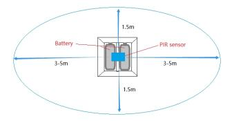
The longer detection range of the motion sensor is in the direction of the side of the battery.
