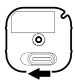
2. Insert two CR123A lithium batteries orientated according to the diagram within your sensor. Try inserting the batteries flat rather than at an angle.
