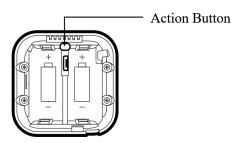
3. If reset successful, the blue led will fade in and out to indicate it is ready to be paired to a new hub.
