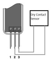
You can wire any dry contact sensor output to Terminal #2 and #3 (it doesn't matter which terminal is wired to where). Dry contact terminals are only looking for Open/Close control which will have Door / Window Sensor 7 report its status depending on the state of the dry contact output to Door / Window Sensor 7.
