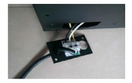
2. Attach the wiring to the junction block. Please make sure the live wire goes into the "L", the neutral wire into "N" and the ground wire into "G".
