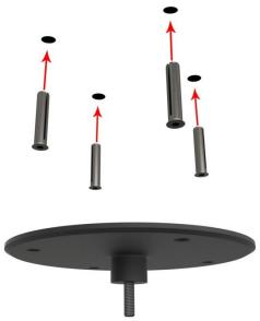
**STEP1** - Mark and drill 4 holes into the load bearing surface and insert the corresponding metal anchor dowels into the holes (anchor dowels are not provided). The holes in the Fixed Ceiling Base are Ø7mm.
