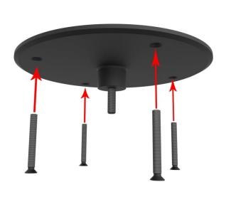
**STEP 2** - Secure the Fixed Ceiling Base to the load bearing surface using steel screws or bolts, depending on the structure it is being secured to (anchor dowels are not provided). The holes in the Fixed Ceiling Base are Ø7mm.
