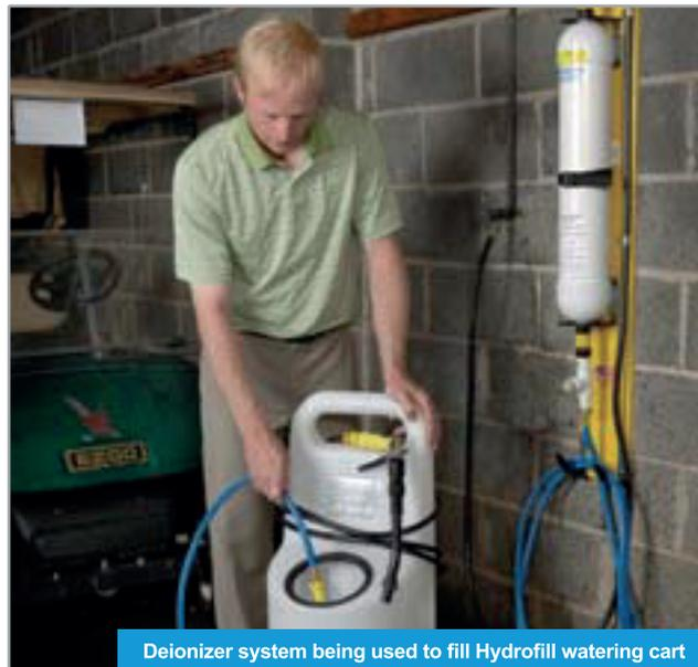
Deionizer system being used to fill Hydrofill watering cart
