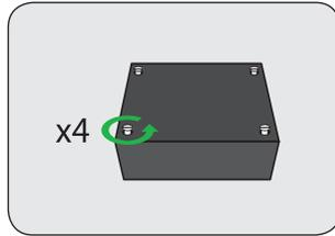
Remove the 4 screws from the battery case.
