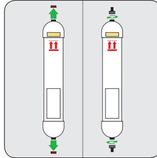
Remove the red caps from the cartridge and thread on the 2 male quick-connect fittings.
