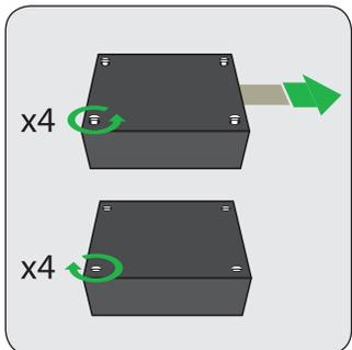
Loosen 4 screws of battery case and pull out tape to activate. Re-tighten screws.
