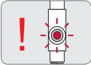
Red flashing light = Replace cartridge.
