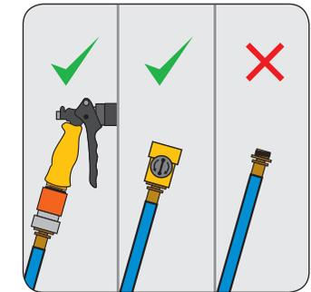
Attach either the **Watering Gun** or **Flow Restrictor** to the free end of the blue hose.
