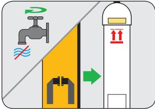
Ensure water supply is turned off and remove cartridge.
