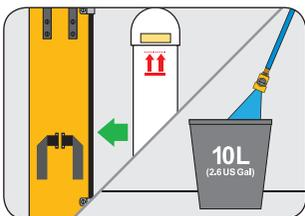
Fit new cartridge and run off 10L (2.6USGal) of water before use.
