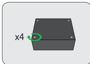
Replace the 4 screws in the battery casing.
