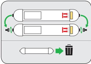
Transfer the 2 male quick-connect fittings to the new cartridge then safely dispose of the old cartridge.
