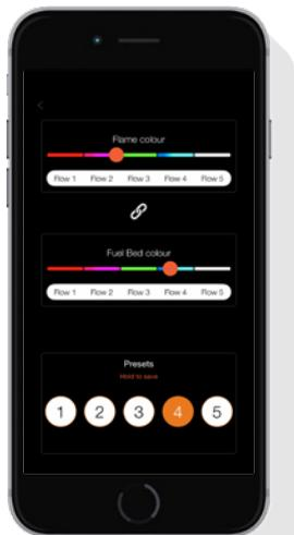
**NB. The fire will retain the last dimmer and colour set by the remote or the app unless the fire is switched off by the master on/off switch, then it will default back to: Flame – Orange 3 Fuel – Flow 5**
