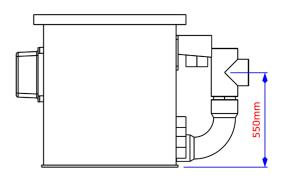
As extra protection, the 2 plugs of the top plugged holes can be removed so that the water flows further unfiltered during an emergency and there is no risk that water is pumped directly into the rinse duct.
