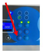
If you keep this button pressed, the pond pump will stop and the motor and rinse pump will be activated. When you release it, the system will turn off. Then press the AUT buttons again (green light will turn on again) to reactivate the system (pond pump will turn on again).
