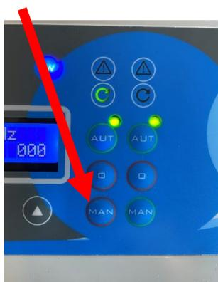
If you keep this button pressed, the pond pump will stop and the motor and rinse pump will be activated. When you release it, the system will turn off. Then press the AUT buttons again (green light will turn on again) to reactivate the system (pond pump will turn on again).
