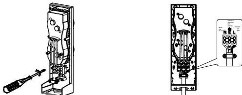
4. Install and tighten the socket into the four customized holes by screwdriver.
