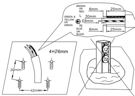
3. Remove the cable anchor from socket outlets by screwdriver, put the wire through the hole at the bottom of the socket, tighten and connect the "L", "N" and "E" terminal corresponding by screwdriver. Install the cable anchor on socket outlets again and make sure the wire is pressed tightly.
