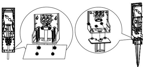
5. Insert the cover plate into the socket and pass the grounding wire through the clamp groove of the cover plate. Do not press the wire and lock it with two screws. Insert the socket into the cover and tighten the product with six screws.
