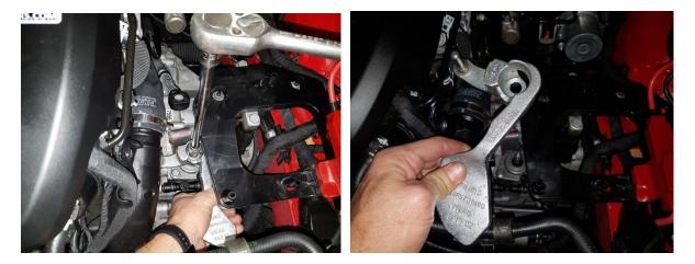
The bottom black shift cable connector must moved backwards about 7mm which is very easy: Pull back the secure ring (see picture), and pull the connector 7mm backward. Let go of the ring and check if it came back in it's original position.
