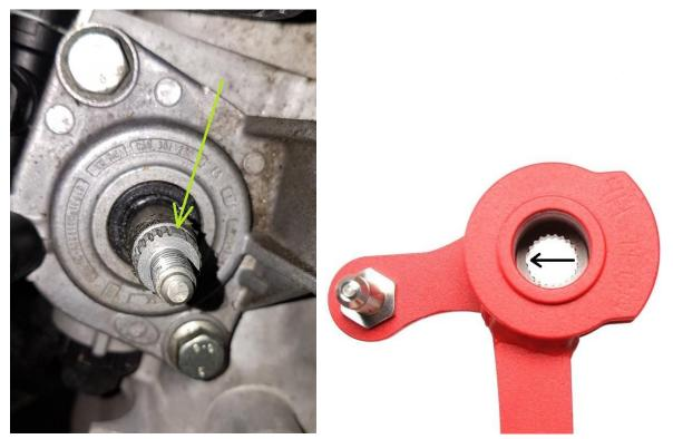
Use the new M8 nut (supplied in the kit) to fasten the 4H-TECH Shifter arm to the gearbox shaft. Tighten the bolt firmly (23Nm), and close the hole with the new dust cap. (self secured cap)
