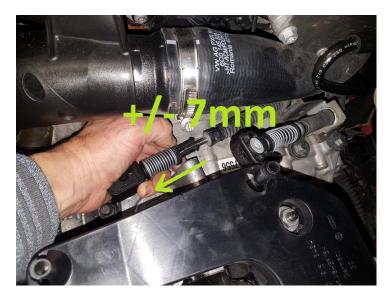
**Important!** The standard shift shaft from the transmission has a splined top. The new shifter arm can only be fitted in **one position**. There is one bigger spline, which must be allined with the **bigger spline** in the shifter arm. These splines have a very tight fit to avoid any play. The best way to fit this is by positioning the shifter arm in the correct position on top of the shaft, and press it manually by hand further on the shaft. Do not use any force here.
