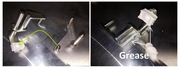
Fit the selector arm in the car, but insert it now from the other side. See picture. Fit the stainless secure ring which is provided in this kit.
