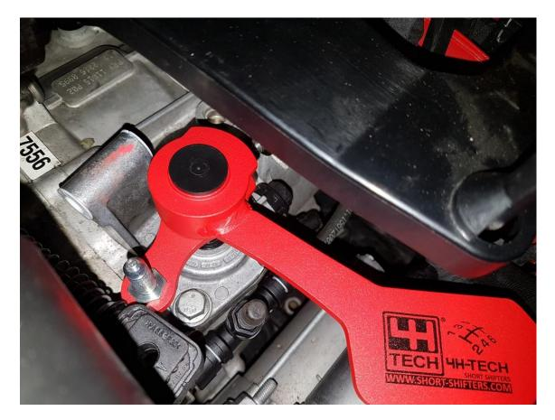
Remove the white slider from the old selector, and put it on the new selector arm. Grease everything up for smooth shifting.
