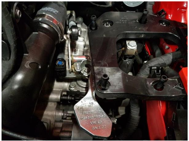
Put the shifter in neutral (don't engage any gears) and remove the 2 clips which hold the shift cables in place, and remove the shift cables from the OEM Shifter system.
