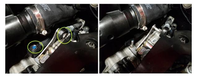
Remove the clip from the selector shaft, and remove the old selector:
