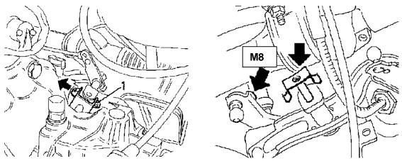
Dismantle the old linkage complete and reassemble every part on the new linkage (shift shortener) When reassambling, fill everything with silicone grease before fitting to be sure of a smooth gearchange.
