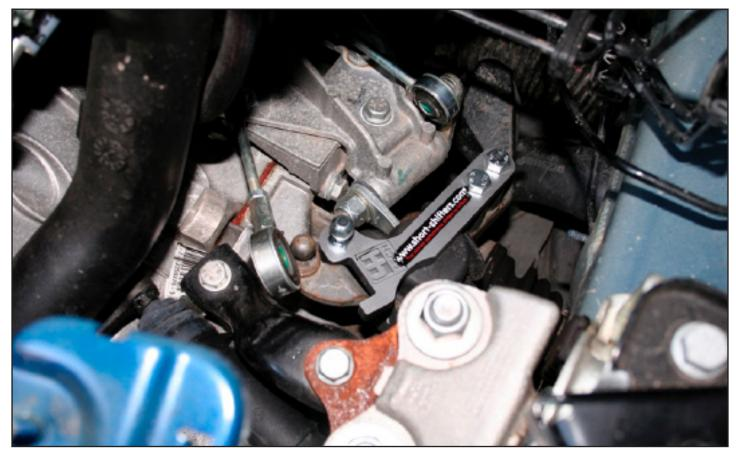
Fit the 4H-Tech Short shifter on the OEM shifter. Important: Support the shifter again while tightening the 2 M8 bolts so no forces reach the inner gearbox.
