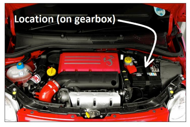
Remove battery, battery housing and ECU
