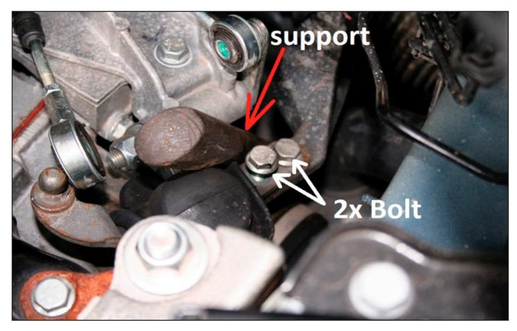
Remove the two M8 bolts. Important: support the shifter with a piece of wood so no forces reach the gearbox.
