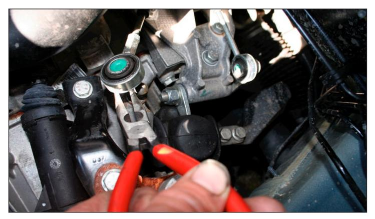
Unlock shift cable from ball joint.
