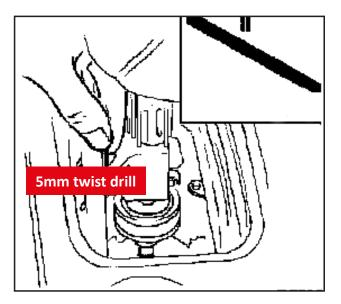
Push the adjustment pin in the gearbox casing. (Turn the selector rod protruding from the selector cover in an anti-clockwise direction (looking towards the front of the car) until the adjustment pin will slide onto it.
