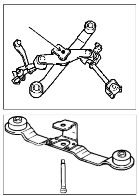
**Dismantle the old linkage complete and reassemble every part on the new linkage (shift shortener)** When reassambling , fill everything with silicone grease before fitting to be sure of a smooth gearchange.
