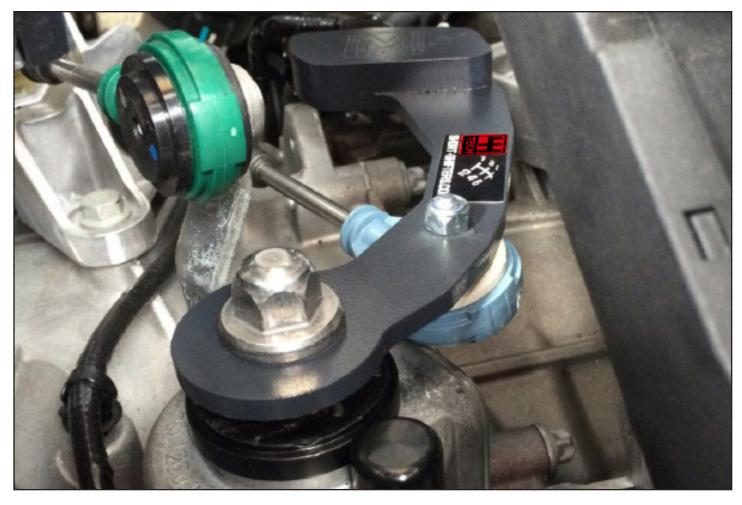
Click on the shift cable first, before mounting the shifter. Thighten the nut very firmly with one hand, while supporting the shifter with your other hand. No re-adjusting neccesary.
