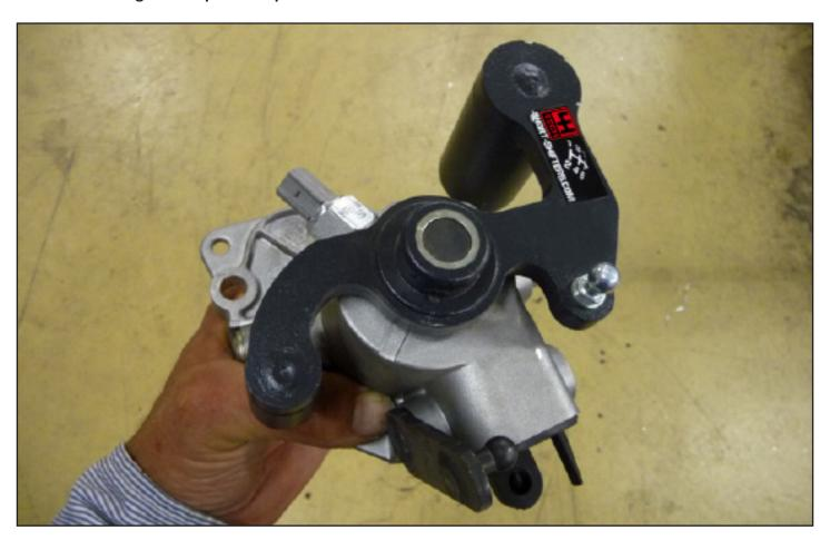
Build the shifter unit back on the gearbox, connect the sensor back on, and click the shift cables on the shifter arms.
