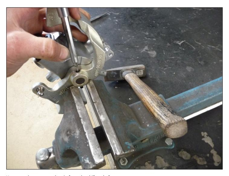
Use a punch to remove the pin from the shifter shaft.
