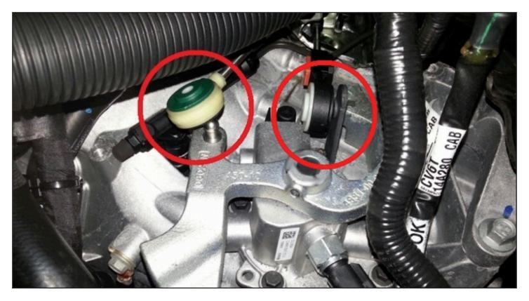
Unclip both shift cables by putting a 13mm spanner between the cable head and the shifter arm.
