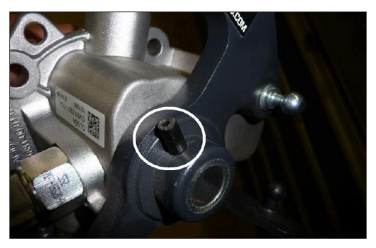
Use the old pin to secure the new Short Shifter arm to the shaft of the shifter unit. You can use the punch and a hammer again to tap it in to place.
