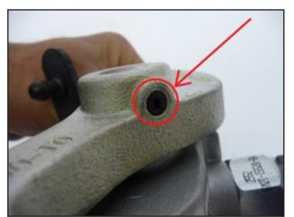
The original shifter arm is secured on the shaft with a steel pin. This pin can not be removed with the shifter still in the engine bay. For this reason it is neccesary to remove the complete shifter unit.
