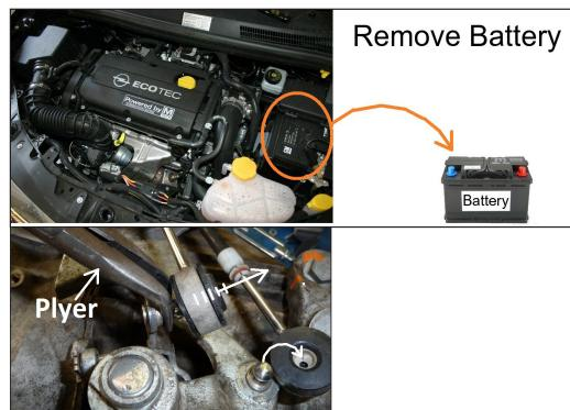
Remove cables from ball joints.
