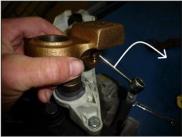
Remove the shift cable on the left side of the shift linkage by using a 11mm spanner as leverage. Pull up the shifter arm and tillt it to undo the shift bar from the gearbox selector arm.
