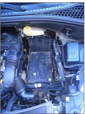
Remove the battery tray and remove the second (metal) battery tray . (M8 bolts) The following pictures are showing the gear linkage out of the car to make things clearer to see:
