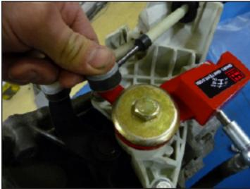
Tighten the bolt on top of the shifter, and click the left shift cable on the new shifter.
