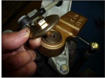
Look at the white plastic bracket where the original shift linkage is mounted on. Remove the big top bolt securing the shifter to the white bracket. (second picture)
