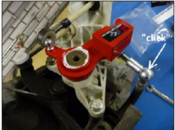
Fit the original ring to the short shifter and put it on the bracket. Click the shift bar on to the selector arm, and secure it with the second pin.
