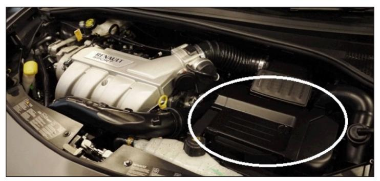
Open the bonnet, and remove the air intake hose, air filter housing and battery . Unclip the front- and rear connectors from the battery tray. Unbolt the battery tray from the chassis.
