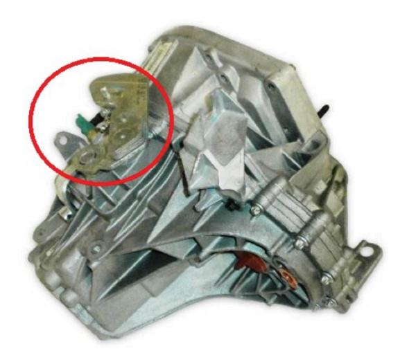
The following pictures are made from the gearbox removed from the car to make the fitting of the short shifter much more clearer to see:
