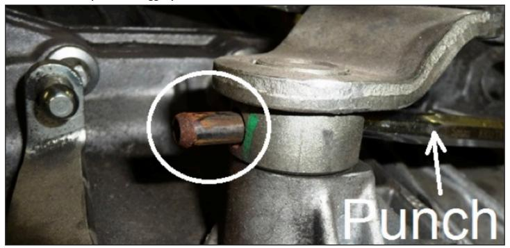
Remove the shifter arm from the transmission:
