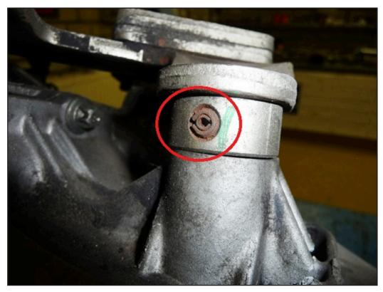
The inner pin must be removed first:
