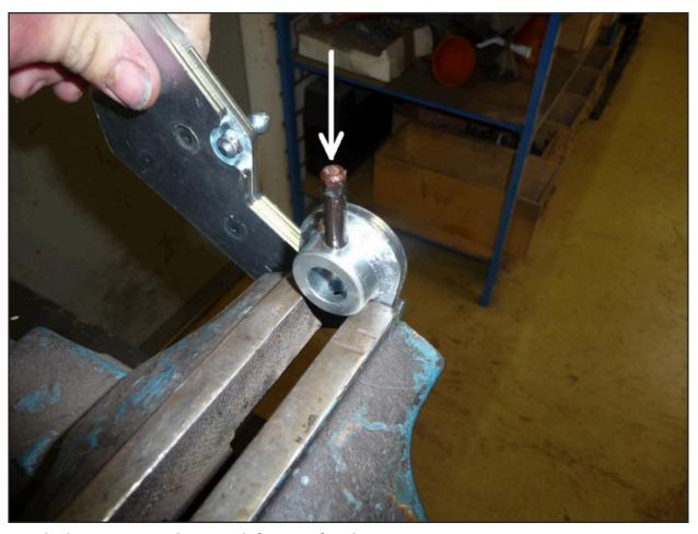
Tap the large pin in to the new Shifter arm for about 4mm.
