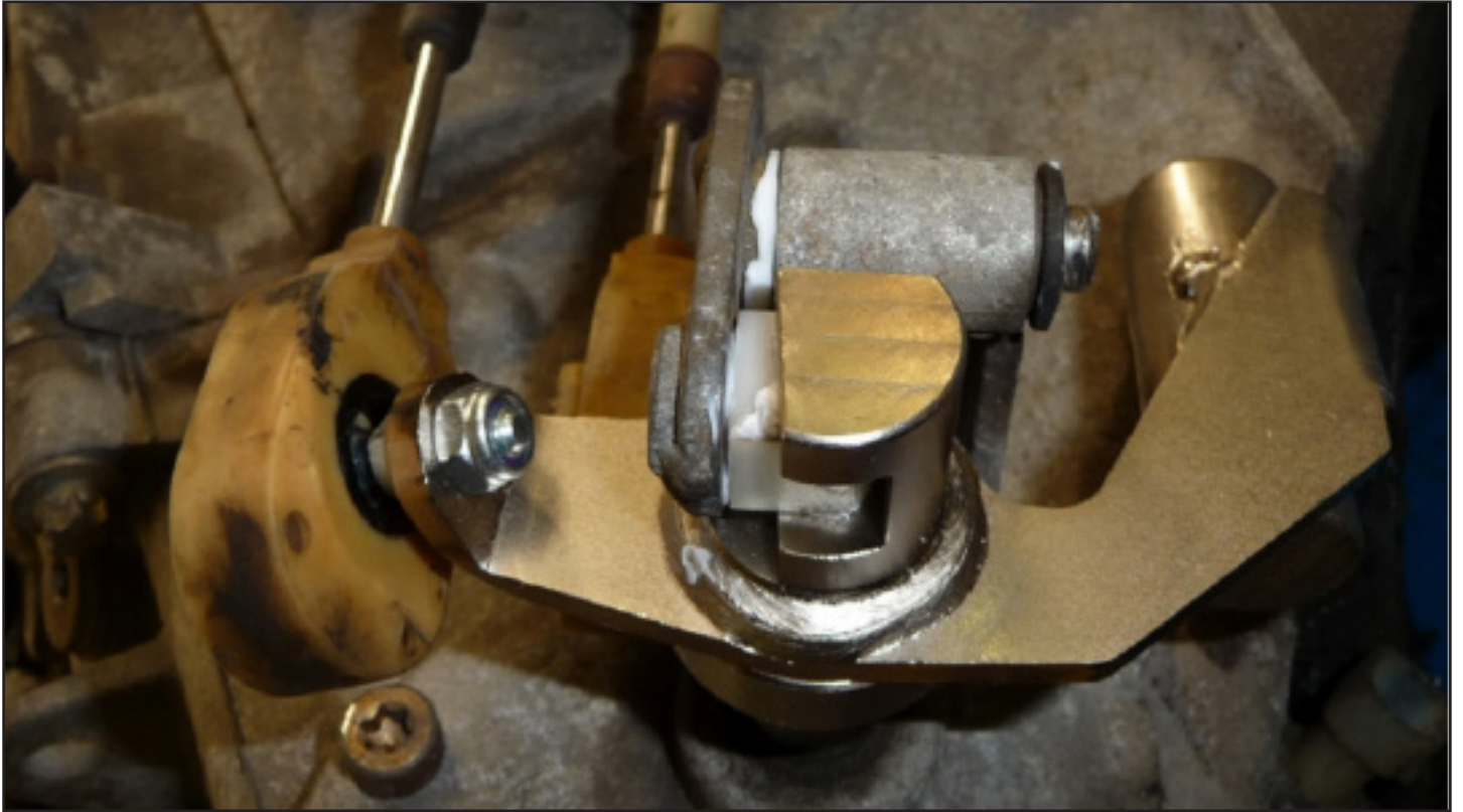
Fitment of stainless steel shift cable re-positioning bracket*:
