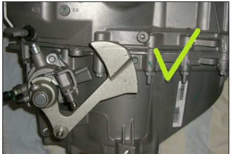
This gear shift shortener will not fit on the gearbox shown in the first picture. See difference in gear lever design.
