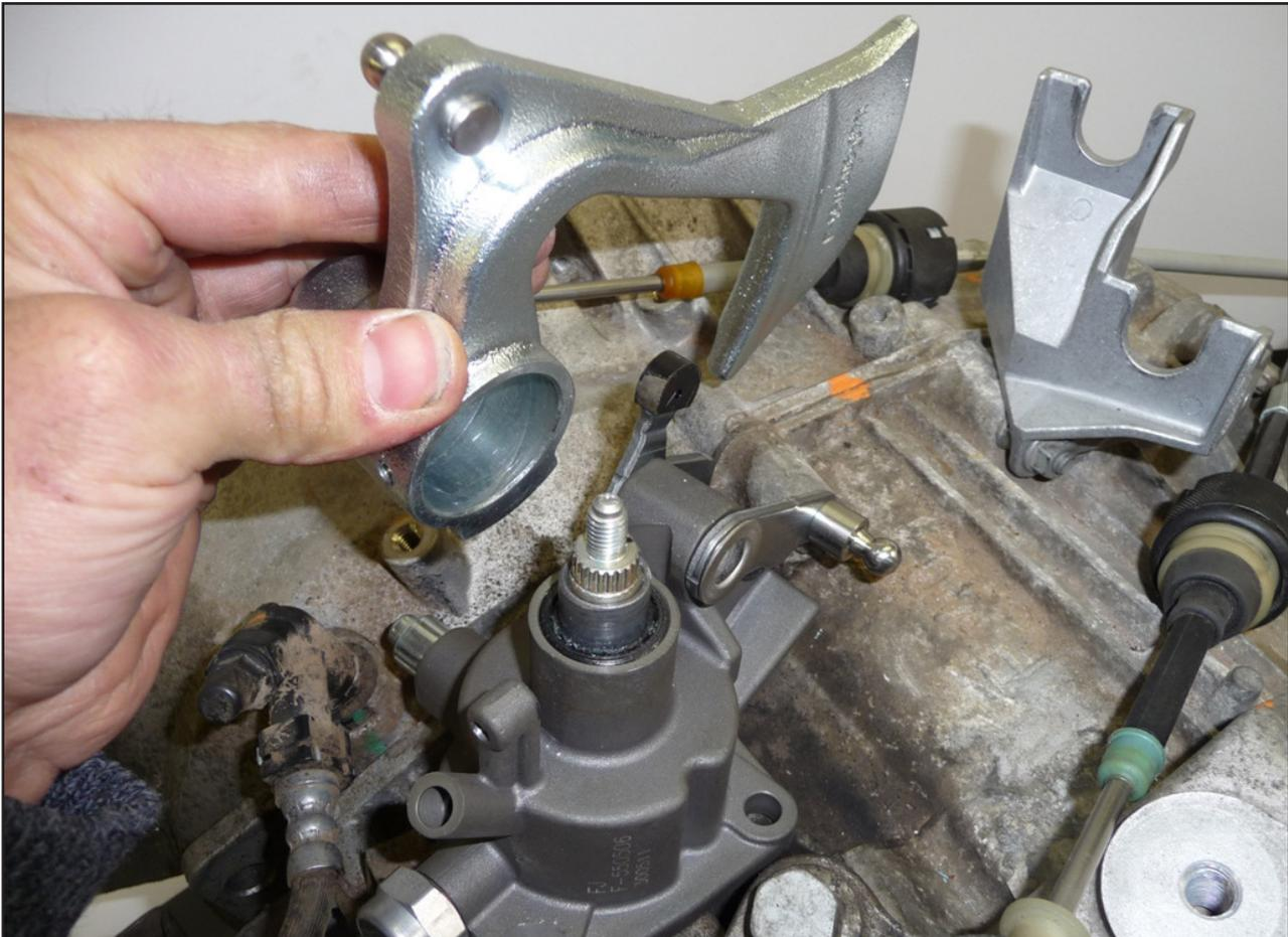
**Important note:** The old linkage can be hard to remove on some old rusty models. Use a pulley removal tool if necessary. Try not to damage the gear shaft. Mostly the old linkage will come off when pulling and wiggling gently by hand.
