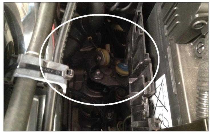
The fitment of the short shifter can be taken place with only removing the ECU of the car and put it aside with wiring still connected. But to get some clear pictures for this fitting guide, we have removed the battery tray in the following pictures.
