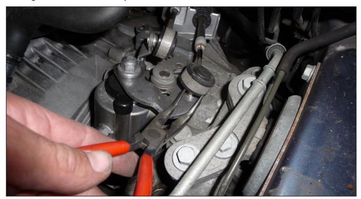
Remove Top nut. Important: support old leaver with your hand while removing the nut!
