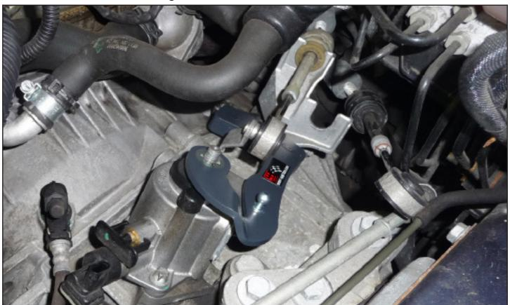
Thighten the nut very firmly with one hand, while supporting the shifter with your other hand. Push the shift cable back on the ball head. No re-adjusting neccesary.
