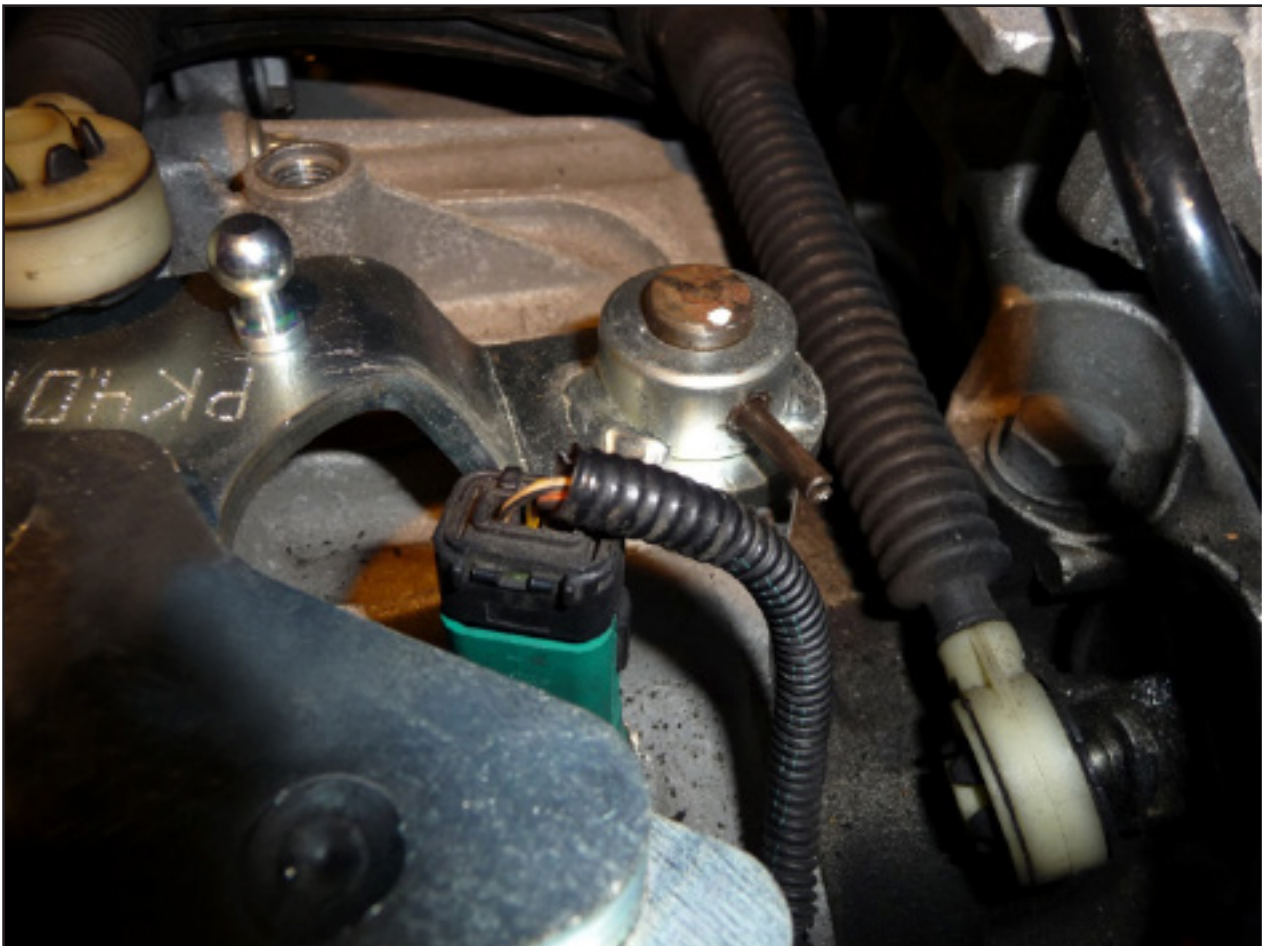
Take the inside pin and press it in the outer pin, again with some pliers.
