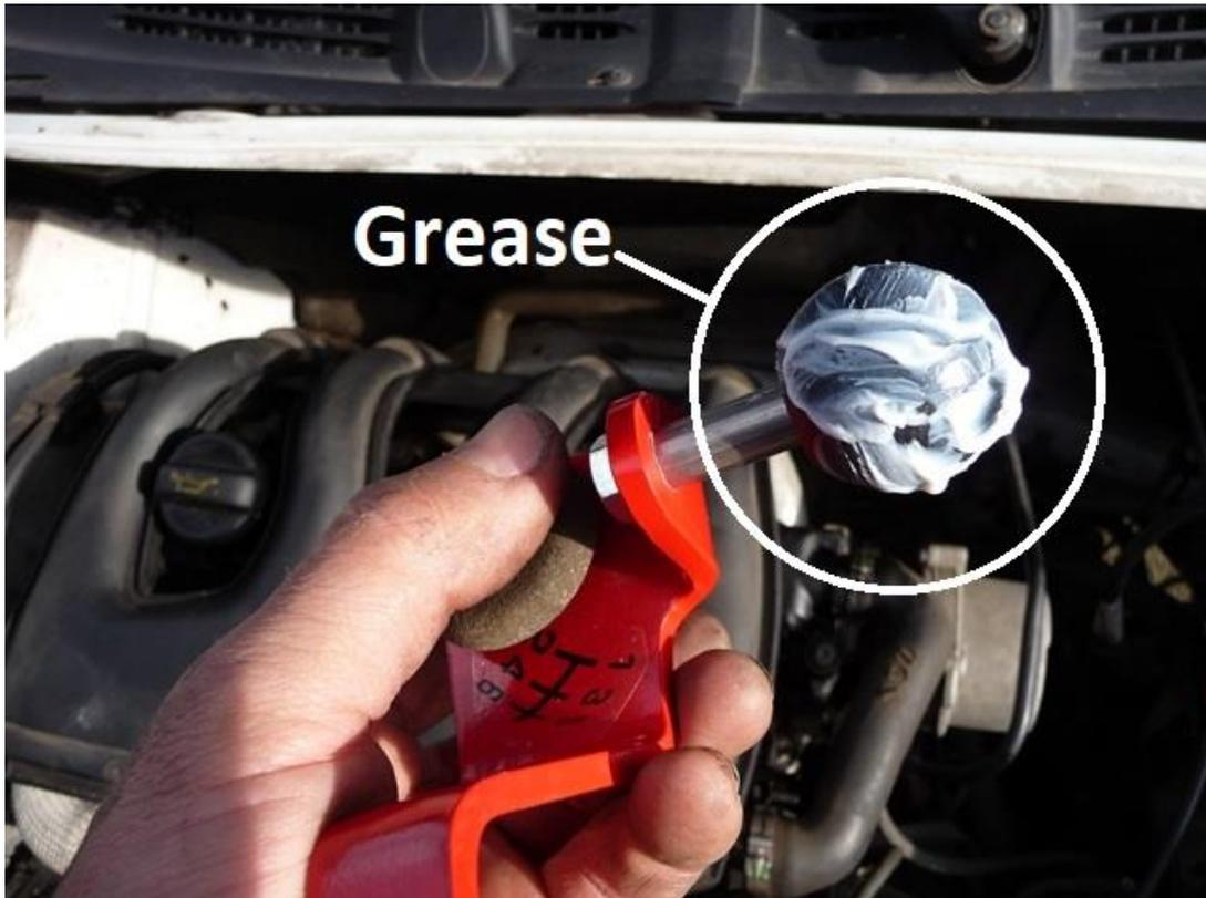
Grease up the new shifter joint, and fit it to the shift mechanism in the engine bay.
