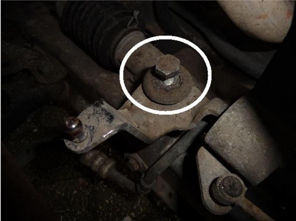
**Unscrew the bolt which holds the OEM shifter. (use 16mm spanner)
