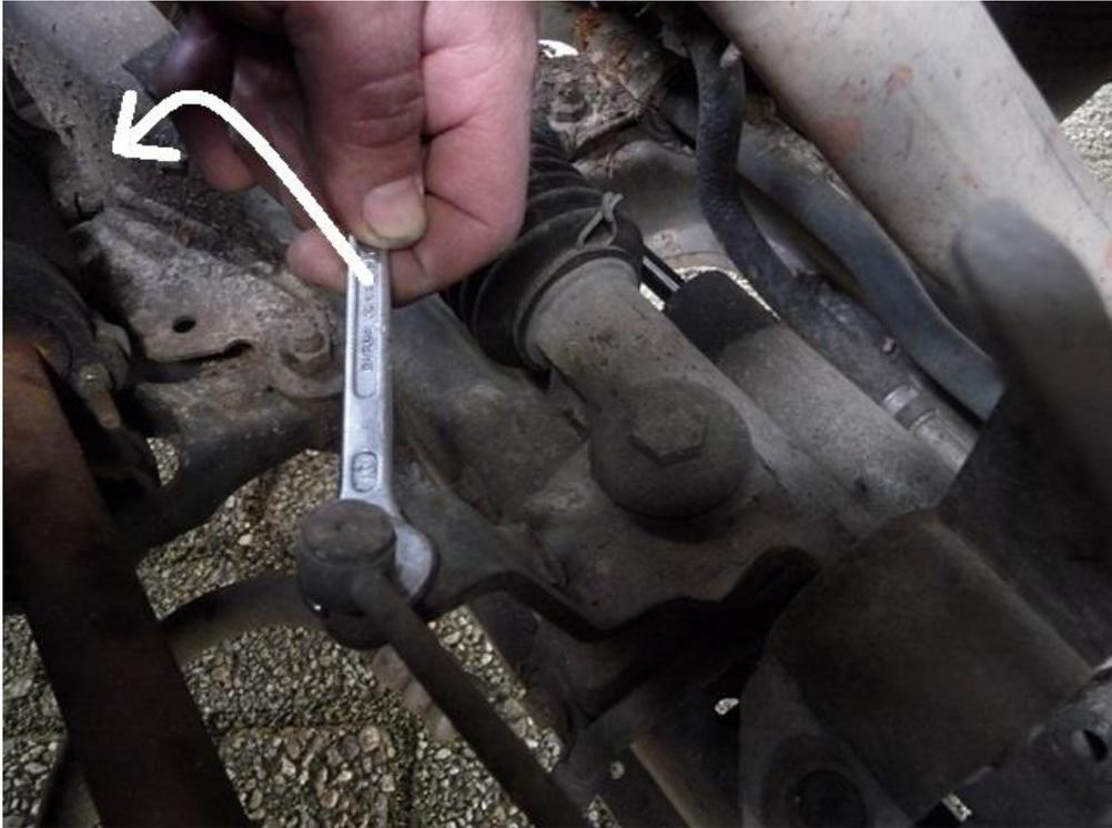
**Use a 10mm spanner to unclip the shift bar from the bolt head.**
