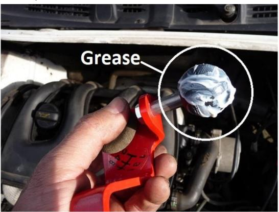
Grease up the new shifter joint, and fit it to the shift mechanism in the engine bay.
