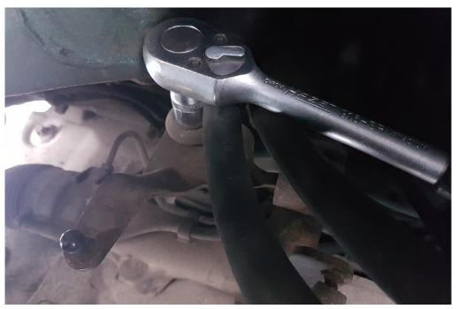
Unscrew the bolt which holds the OEM shifter. (use 16mm spanner) Remove shifter arm and undo it from all components.
