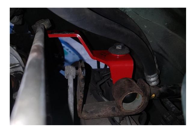
click the shift bar on new shifter by pressing it on the bolt head, and tighten the bolt with a 16mm spanner.
