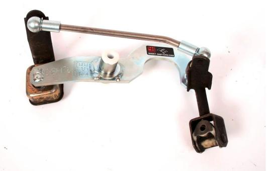
Fit all parts to the new shifter arm, and use the new shifter bar on top, and fit the new nylon bushings
