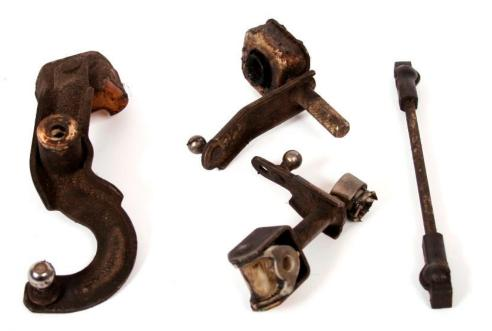
Remove all single shifter parts from the OEM shift linkage.
