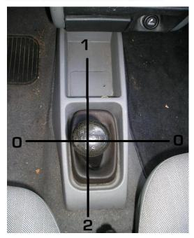
Keep the gear leaver in the neutral position against the left side and keep it in this position. (Line of the first and second gear).
