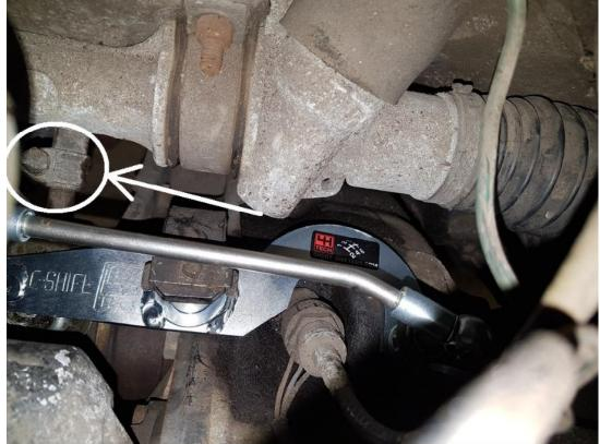
Put the new shifter back in the car. Fit everything in reverse order, but wait with tightening the bolt which connects the shifter with the shift leaver bar.
