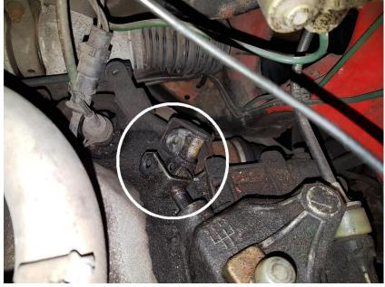
Remove pin between gearbox and shift mechanism
