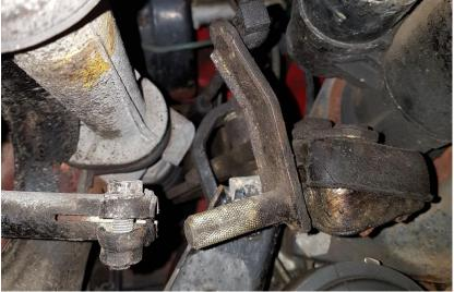
Losen the bolt from the shift bar
