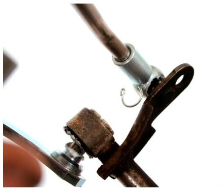
Dong forget to secure the new top shifter bar with the new pins, like shown on this picture. Put the pins in the little holes of the bolt head, and secure them by turning them over the bolt head. (click)
