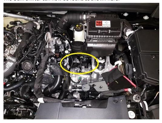
Use a 13mm spanner to remove the shift cable from the OEM shifter arm:
