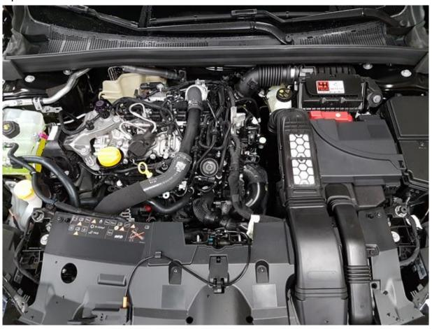
Remove the air filter housing (unclip from the battery tray)
