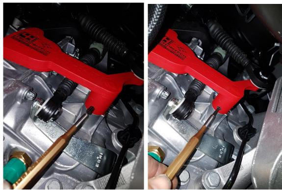
Press the shifter cable on the bolt head from the short shifter.
