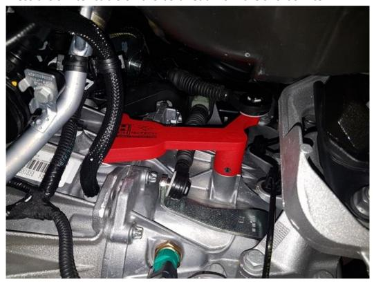
Check if all gear can be engaged with a factory smoothness, and fit all parts back in reverse order.
