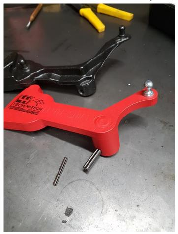
Put the Short Shifter on the transmission shaft and secure it by tapping thebig pin into it first, and the small pin after that. (Both pins can be tapped with the use of the **6mm** cotter pin driver tool. (you can use a 7mm drill if necessary to aline the holes from the back side of the shifter)
