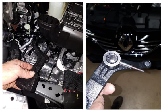
Remove the 2 pins from the OEM shifter and tap the big pin about 4mm in the 4H-TECH Short shifter as shown on the picture:
