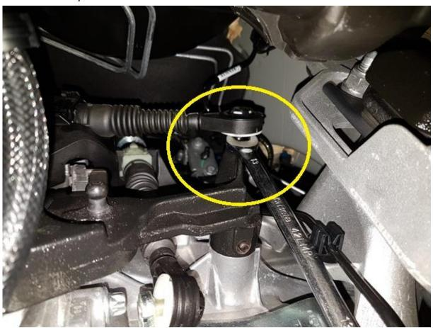
Unclip the connector from the transmission:
