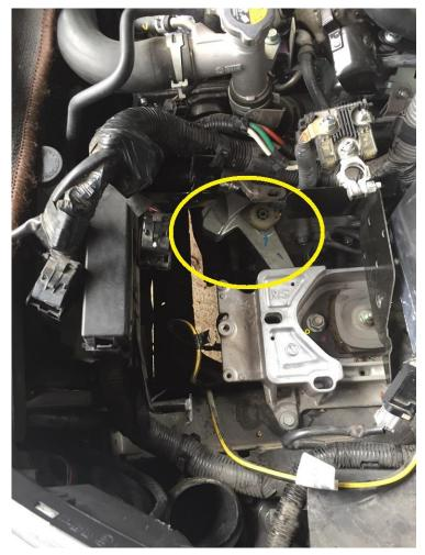
Use a 13mm spanner to remove the shift cable from the OEM shifter arm:
