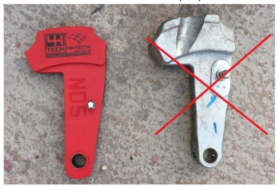
Put the new Short Shifter arm on the shaft, and secure it with the original pin. Click the shift cable back on the bolt head of the new shifter.
