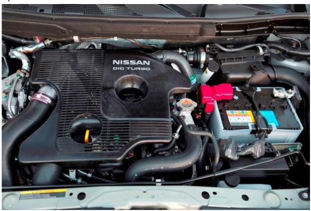
Remove positive and negative battery cable
