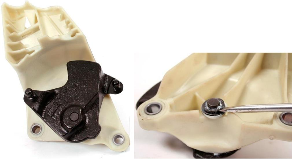
Remove the retaining clip with the use of a screw driver like shown in the picture. Keep the rings which came from the shaft of the old shifter, so you can use them to fit the new short shifter.
