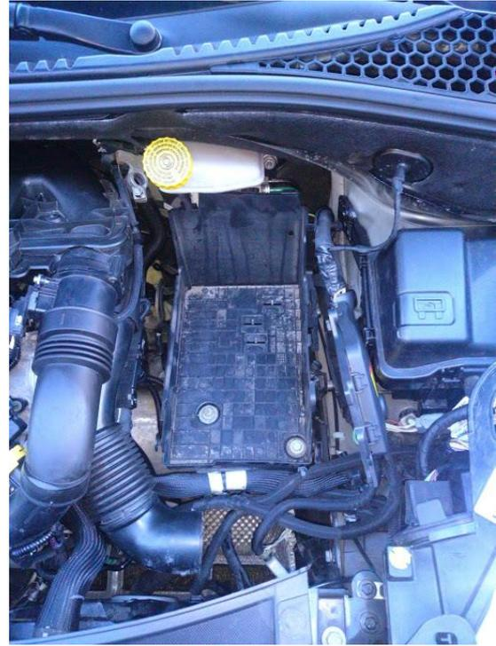
Remove the battery tray and remove the second (metal) battery tray . (M8 bolts)
