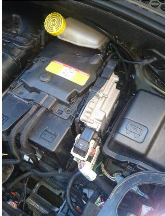
Remove the power distributor on top of the battery and push it to the right side of the battery and leave it there.
