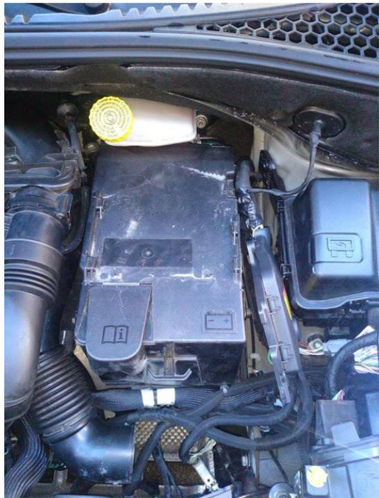
Remove the battery cover and disconnect the positive pole of the battery.
