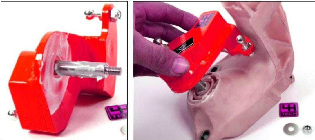
Put Grease on the shaft and the lower part of the short shifter as shown on the picture. (white grease) Fit the short shifter on the bracket, and fit all rings and nuts in the right order back, and secure the shifter shaft with the use of the new secure ring which came with the short shifter kit. (The shifter must be able to rotate freely)
