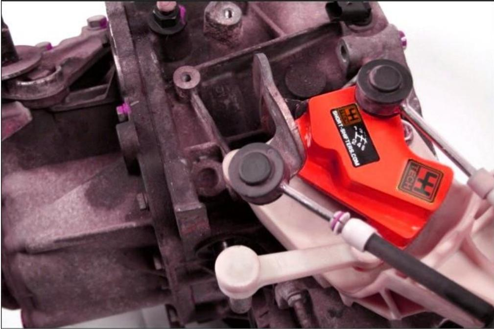
Flip over the plastic bracket again and secure it with the two bolts using a 13mm socket wrench. Secure the underside of the plastic bracket with the nut using a 11mm socket wrench. Put the wheel back on and lower the car.
