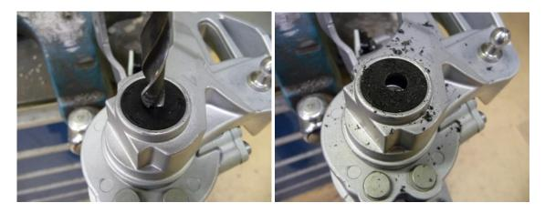
Drill a hole in the plastic cap of the stock shifter
