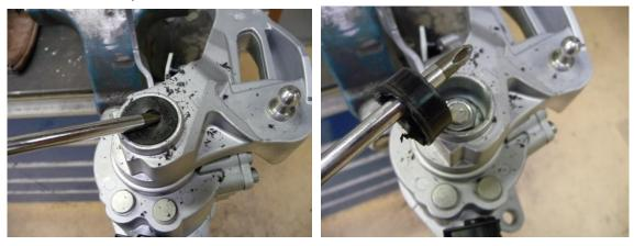
Remove the nut with a 15mm spanner (support the shifter arm with your other hand ):
