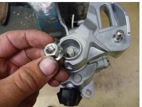
Put the drill (included with the kit) in a cordless drill machine and put the drill over the bolt head of the stock shifter arm. The bolt head will guide the drill. Drill away the aluminium around the bolt head, till the arm comes lose so you can remove it from the shift culom.
