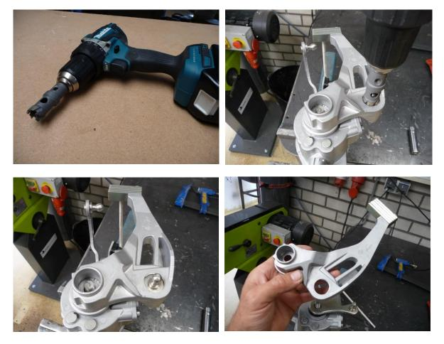
Use the special tool to pull the little metal shifter arm from the shaft:
