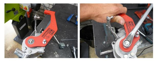
Press the shifter cable on the bolt head from the short shifter.
