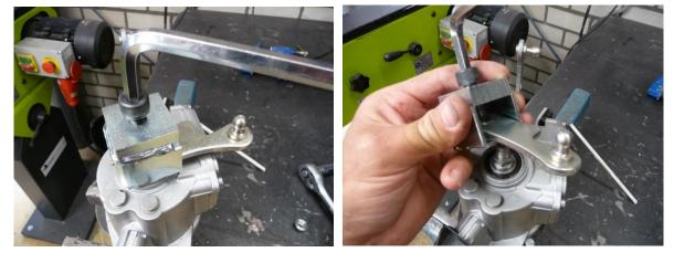
Put the short shifter arm on the hexagon shaft, and push it down the shaft with the nut. Thighten the nut as good as you can, while using your other hand to support the shifter arm. (to avoid putting stress on the shift shaft itselve)
