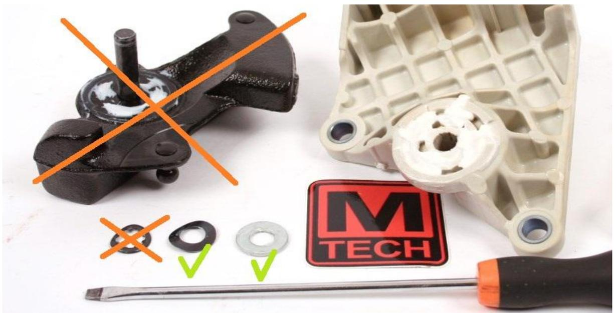
The big ring and the spring ring must be used to fit the new short shifter to the bracket. The retaining ring can be left away, because the new shifter will be fastened with a M6 nut.
