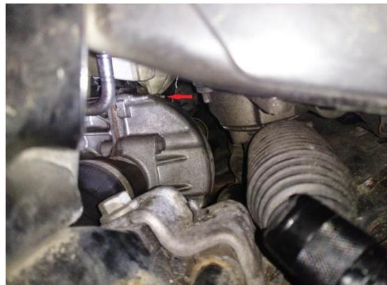
Remove the two bolts on top of the white plastic bracket. And flip the bracket & shift linkage over so you can see the underside.
