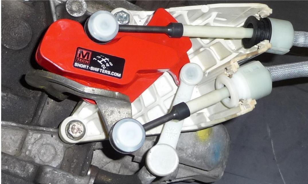
Flip over the plastic bracket again and secure it with the two bolts using a 13mm socket wrench. Secure the underside of the plastic bracket with the nut using a 11mm socket wrench. Put the wheel back on and lower the car.
