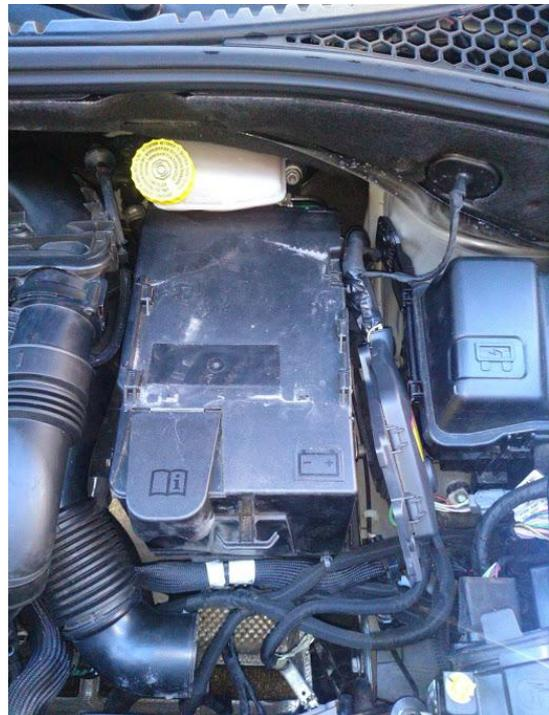
Remove the battery cover and disconnect the positive pole of the battery. Remove the bolt securing the battery with a 13mm socket wrench and remove the battery.
