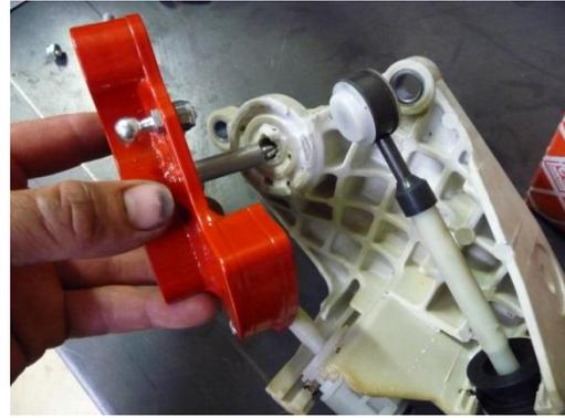
Put Grease on the shaft and the lower part of the short shifter as shown on the picture. (white grease) Fit the short shifter on the bracket, and fit all rings and nuts in the right order as shown in the following pictures. (The shifter must be able to rotate freely)
