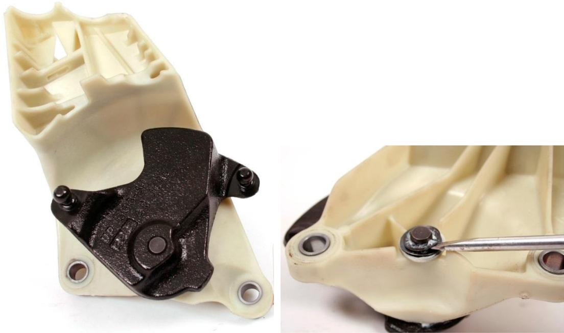
• Locate the original Shift linkage **on top of the gearbox**. Remove this from the car including the plastic bracket like shown on the first picture. Make also very sure your original shift linkage looks **exact like this one** on the picture because different types are existing. (which are used on other Peugeot and Citroën models)
