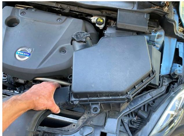
Pull the air filter housing up (from its rubber mounts), and remove it.
