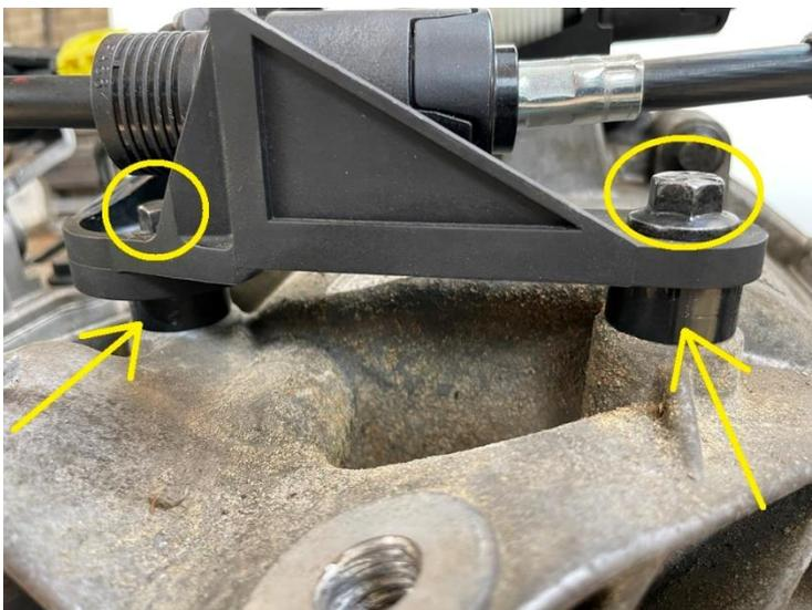
Unscrew the 2x M8 bolts, and put the 4H-TECH Spacers\* between the bracket and the transmission. Re-tighten the bolts.
