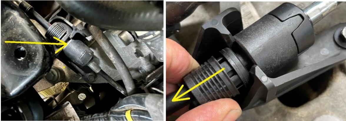
Pull back the secure ring (see picture) and undo the shift cable from the cable bracket.
