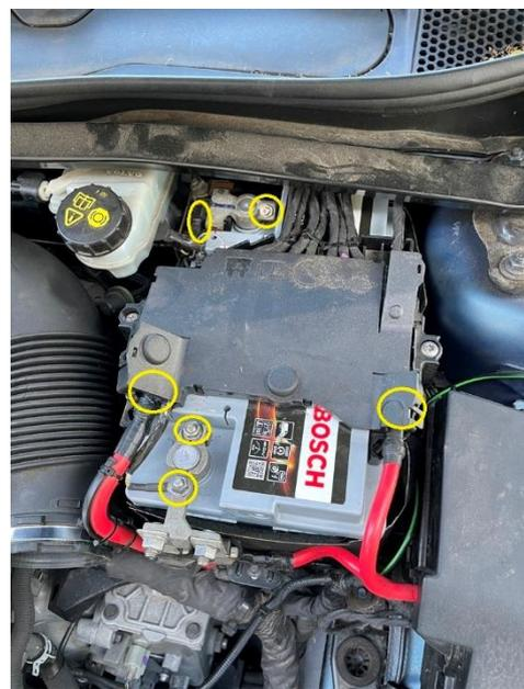
The 12V distribution block can be tilted backwards towards the front window. If you have a Ty-rib, you can fasten it temporary on the wind screen wipers.
