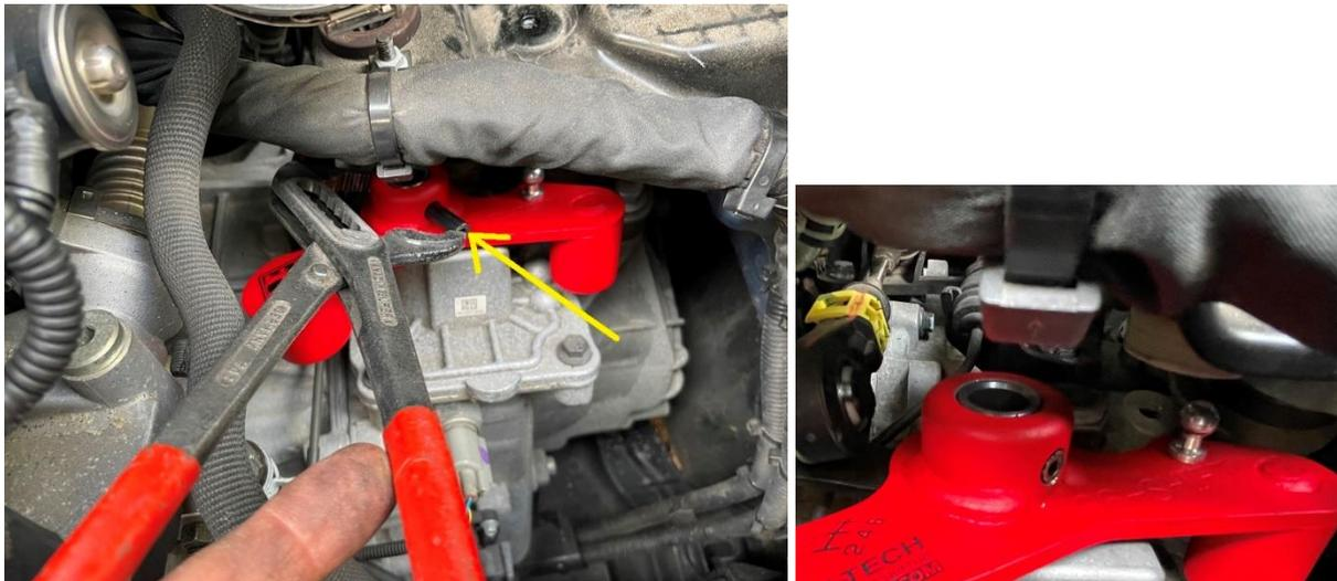
Push the shift cable on the bolt head of the short shifter, and push the plastic top cap on the shifter shaft, to prevent from dirt coming in the shaft.
