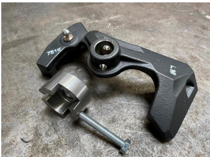
Take the secure pin from the Volvo shifter arm, it can be re-used, and tap it in the 4H-TECH Short Shifter. Tap it in till it is about 1 mm from the head shaft hole.
