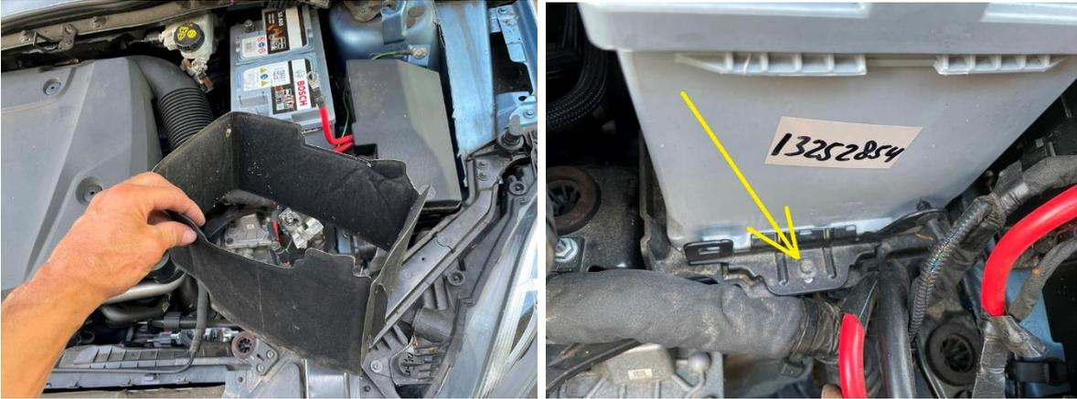
Remove battery and battery tray.
