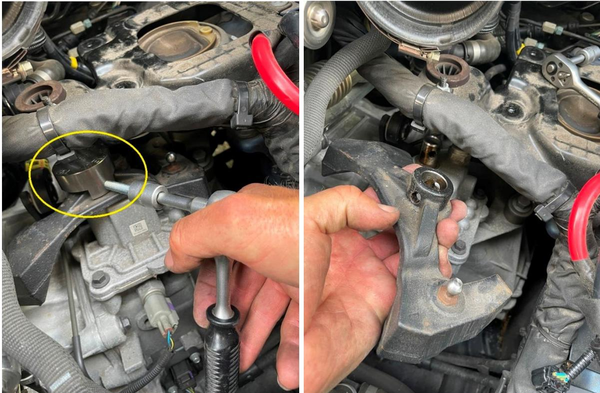
This tool makes the removal of the old Volvo shifter arm very easy.
