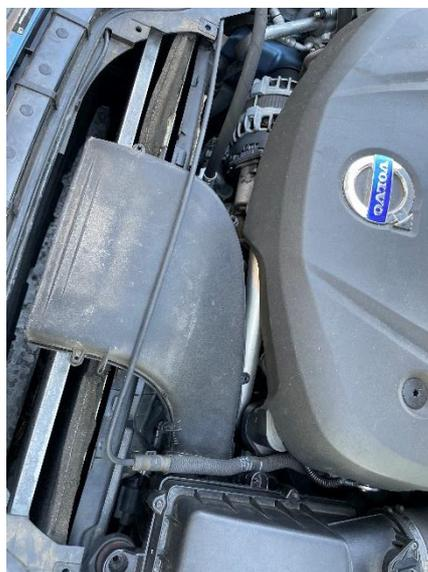
Undo the small coolant line from its fastening points and place it on top of the intake duct, and unclip the line also from the side of the air filter housing.
