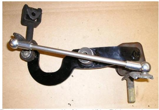
There is a small bent in one side of the top shift bar. This bent must be on transmission side of the car. (left side)
